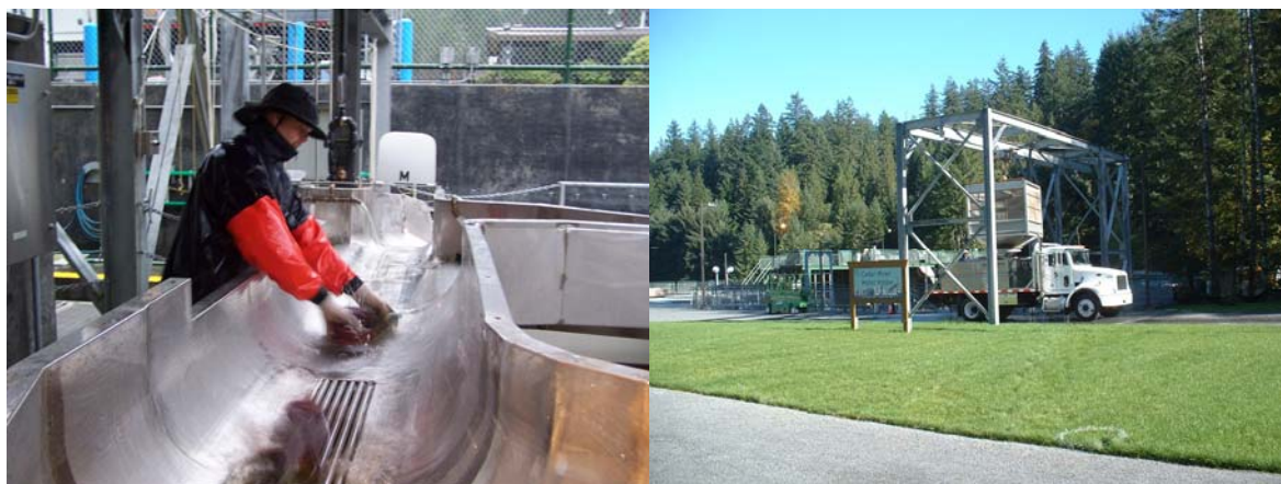
Figure 2: Sorting table operation and fish hopper on top of fish transport truck.
