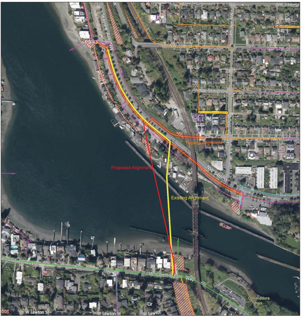
Wastewater Pump Station 43 is located at 5635 Seaview Ave NW in the Ballard neighborhood. It was built in 1958 and serves the NPDES 059 combined sewer basin. Under normal operation, this station has a peak capacity of 4.5 MGD of flow across Salmon Bay directly to King County Metro's Fort Lawton Tunnel via a 1,950 foot long 12-inch diameter cast iron force main.
