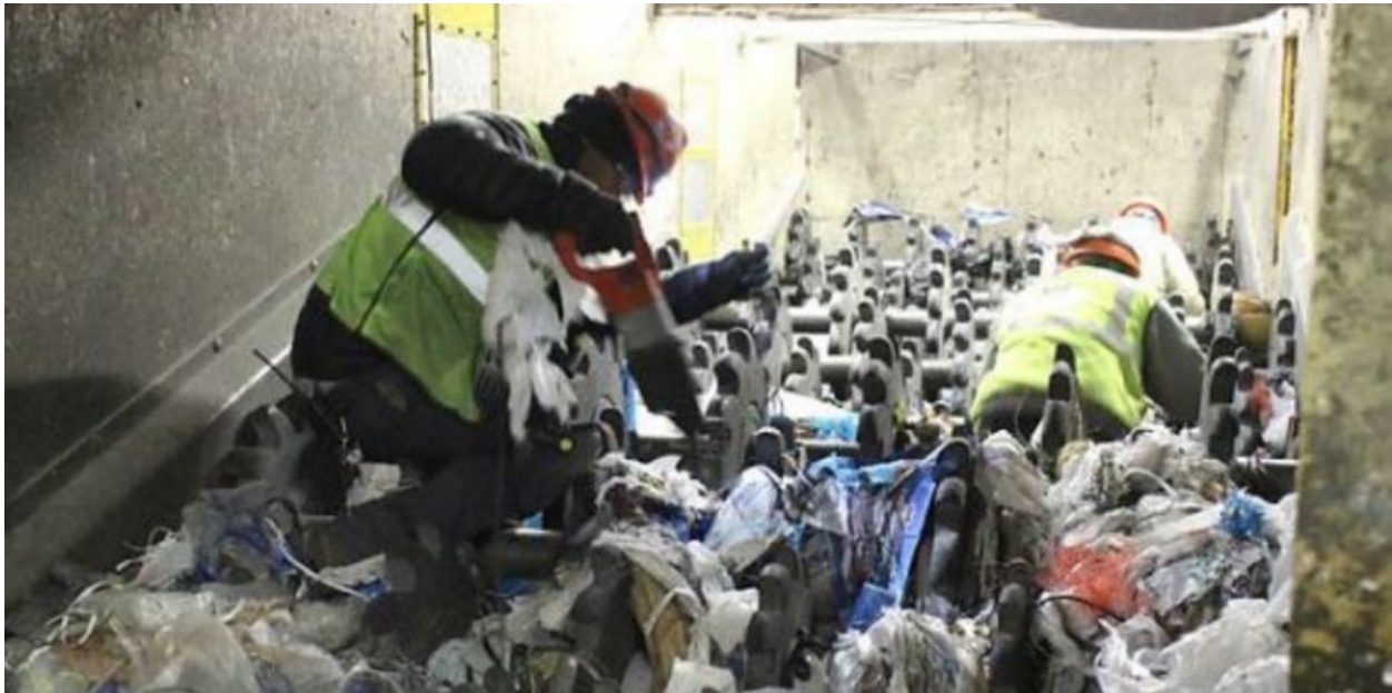
Recycling facility workers cut plastic wrap and bags from sorting screens (Source: SPU 2019 Report on Seattle Bag Ban Compliance)
