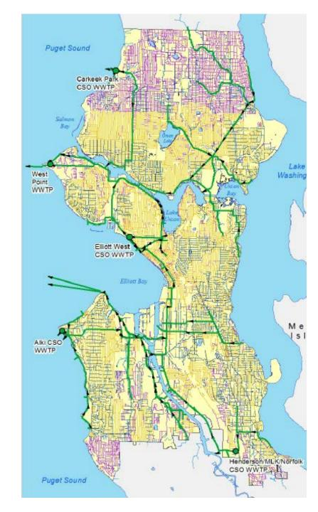
Seattle's Wastewater system includes 68 pump stations and 34.5 miles of force mains.
