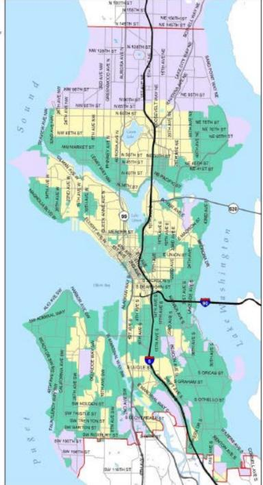
Seattle's Wastewater system is comprised of 475 miles of combined sewers, 379 miles of separated sanitary sewers and 568 miles of partially separated sewers.
