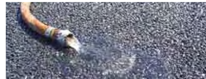
Permeable concrete lets stormwater pass through
