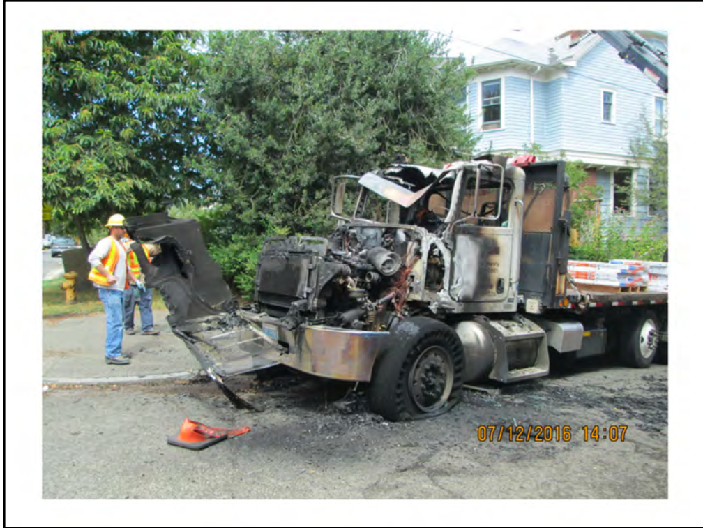
These are images of a boom truck that touched a powerline.
