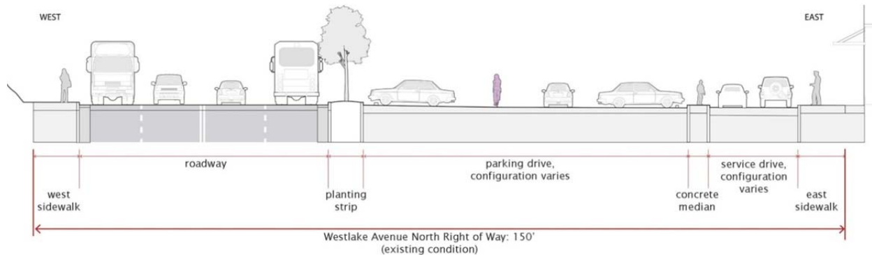
Figure 2. Westlake Avenue North Existing Example Cross Section.
