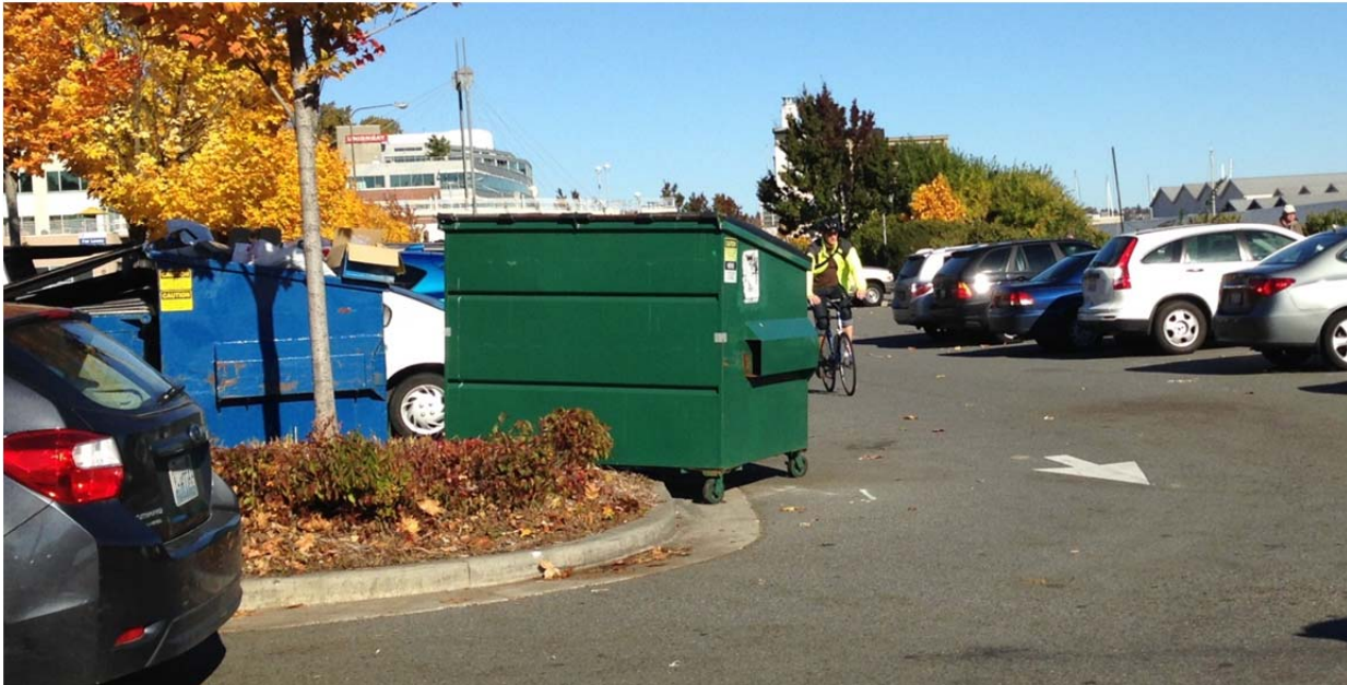
Figure 22. Sight distance limitations for motorists exiting the parking lot onto Westlake Avenue North.
