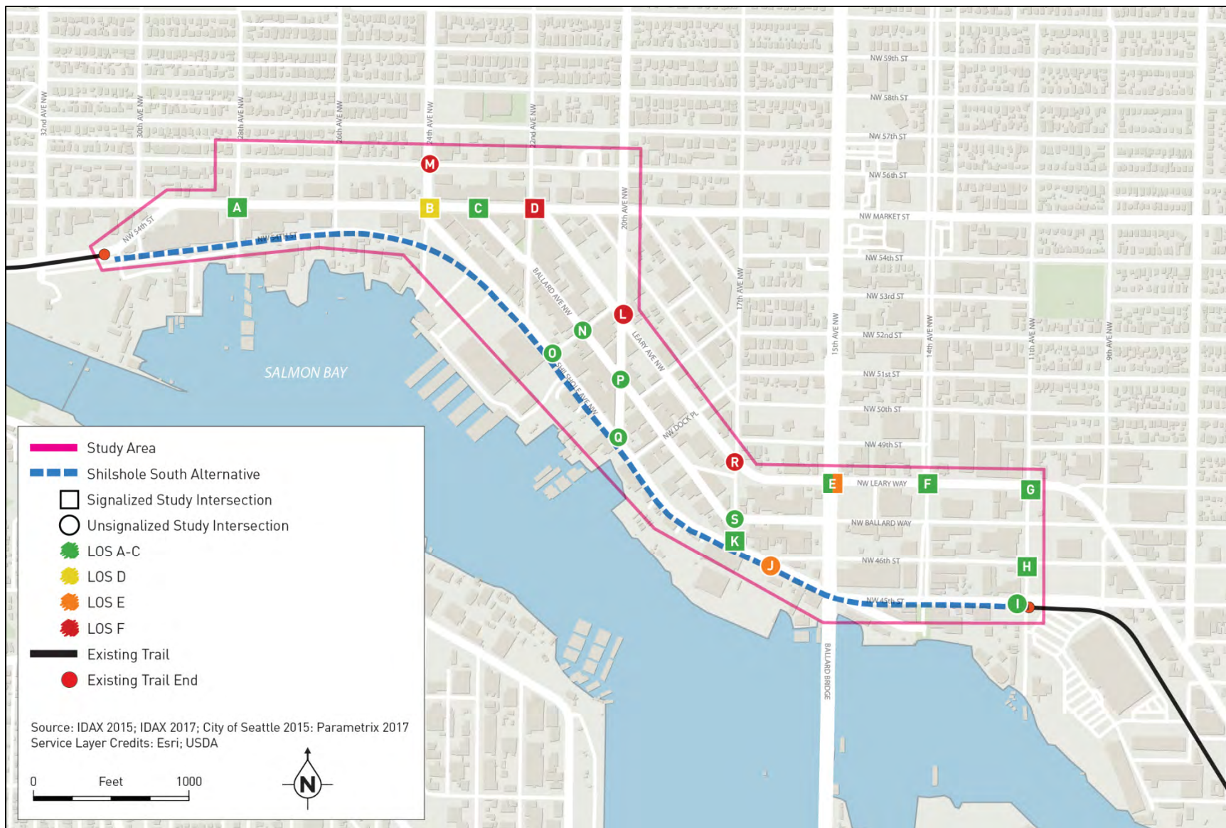
Figure 7-13. Shilshole South Alternative PM Peak Hour Study Intersection Level of Service
