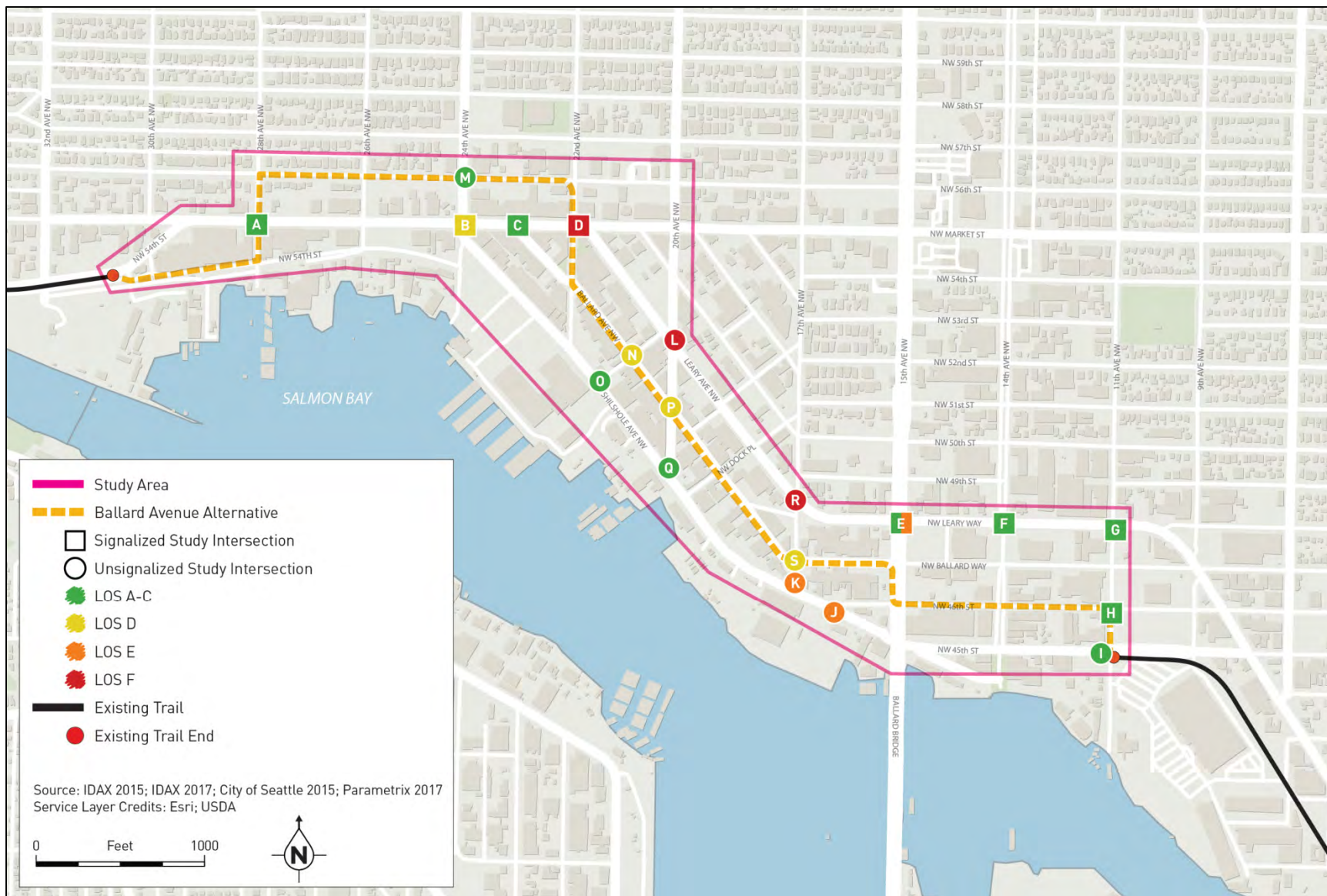
Figure 7-15. Ballard Avenue Alternative PM Peak Hour Study Intersection Level of Service
