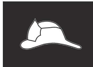
FIGURE 403.6.1.6.5 FIRE SERVICE ACCESS ELEVATOR SYMBOL
