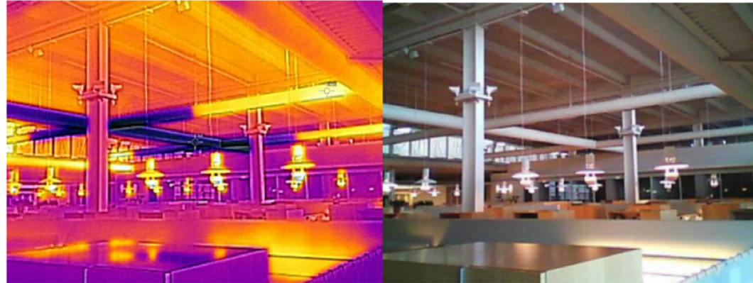
Open Office on Upper Level – VAV's serving same open area operating in both heating/cooling
