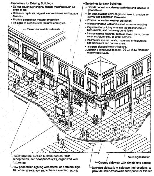
Figure ///-21: Illustration of Design Guidelines Concepts Proposed for The Ave
