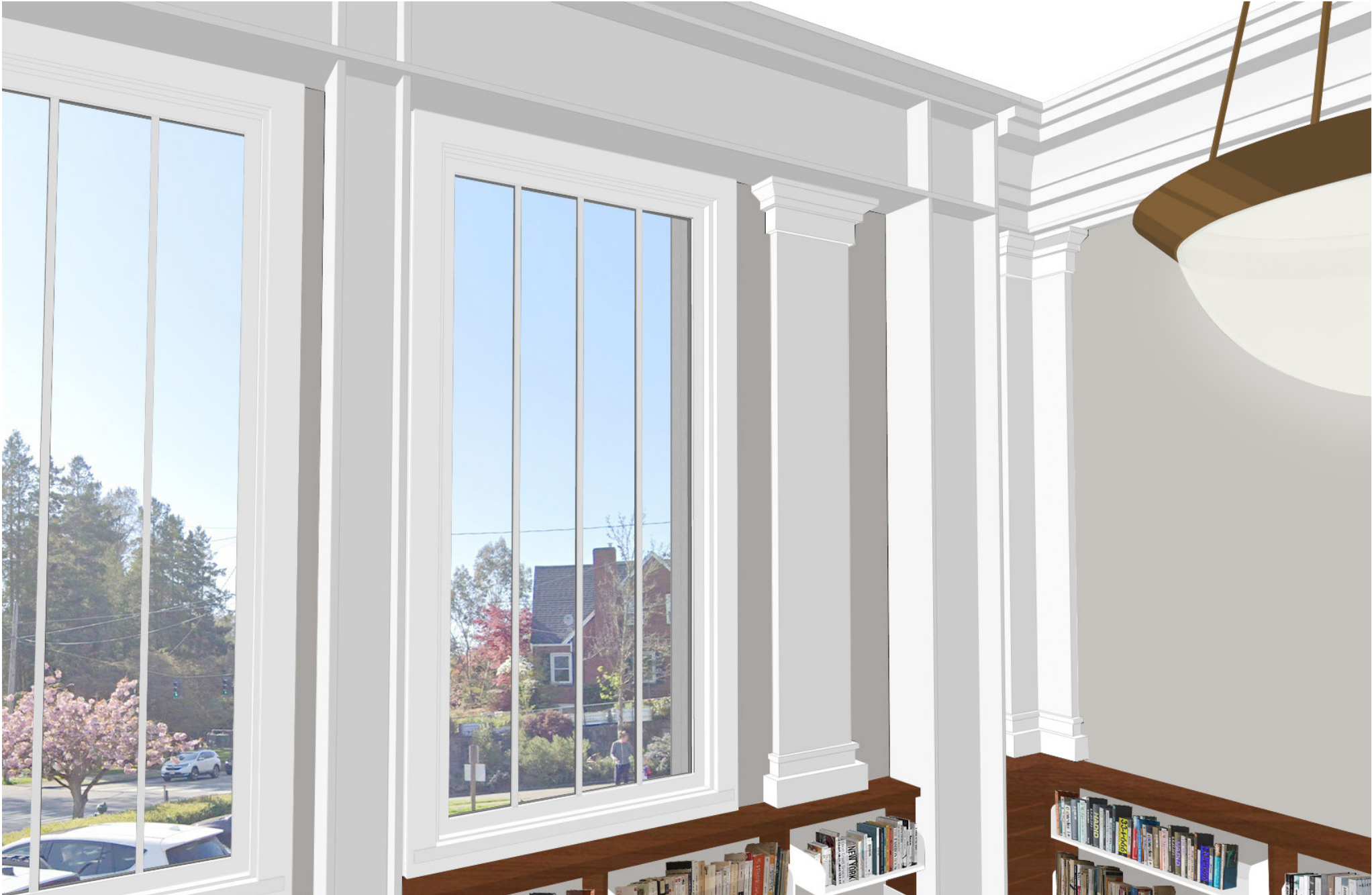
View of proposed moment frame and molding intersection
