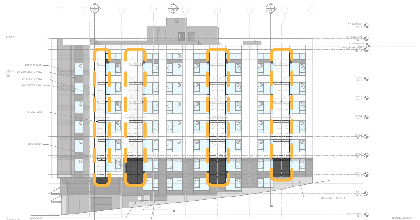
PROPOSED EAST ELEV. W/ VENTS RELOCATED
