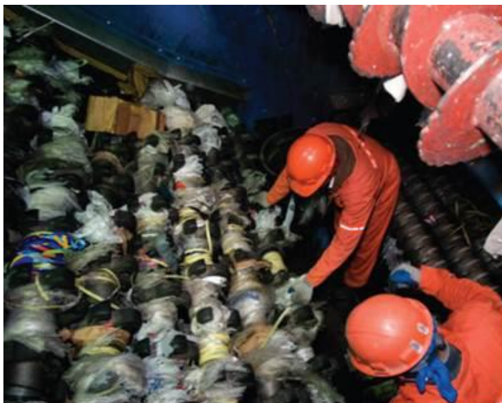
Plastic Wrapped Around Sorting Screens at Materials Recovery Facility
