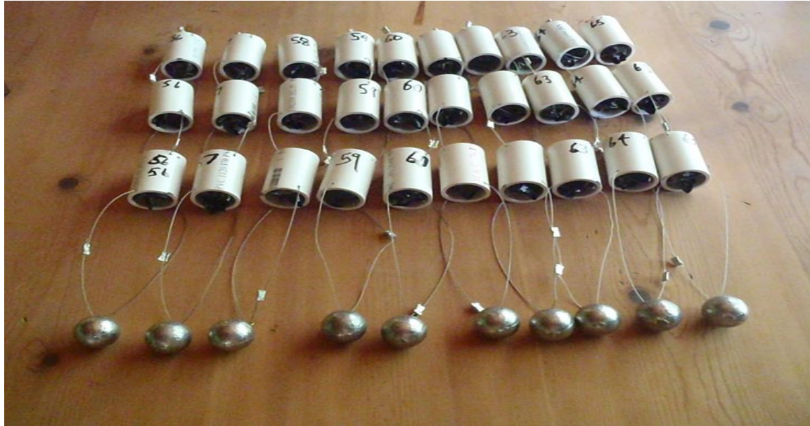
Figure 1. Photograph of 10 fully constructed scour monitors ready for deployment.
