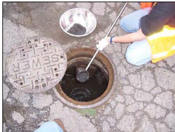
Figure 5: Inline grab sampling
