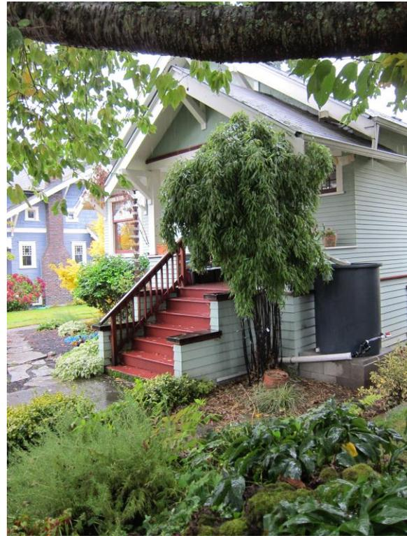
**Figure 4-13. Rain garden (left) and Cistern (right)**
