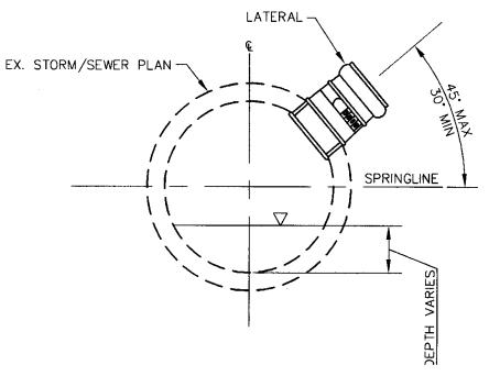
Figure 1 Cross Section Standard Tee
