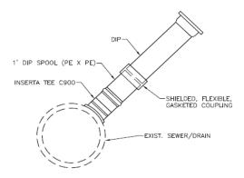
Figure 3 Ductile Iron Lateral Connection
