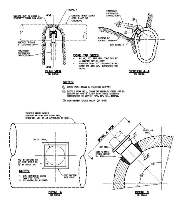
**Figure 5 Connecting to Brick Pipe**
