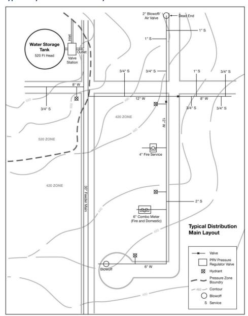
Figure 5-2 Typical Layout of SPU Water System Infrastructure
