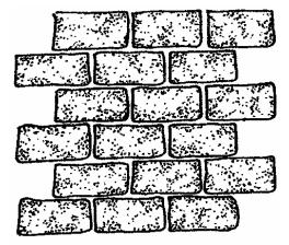
The Contractor shall use the "running bond used brick" pattern for crosswalks or at other locations when shown in the Drawings.
