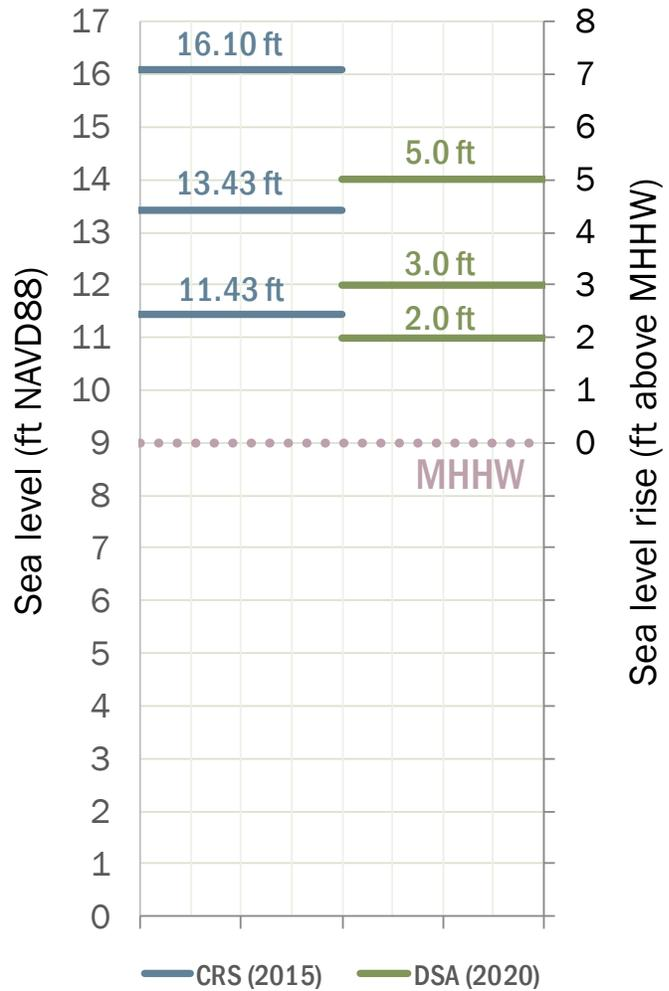
**Figure 3-3. SLR scenarios for this study (DSA 2020) compared with sea levels in the CRS**
