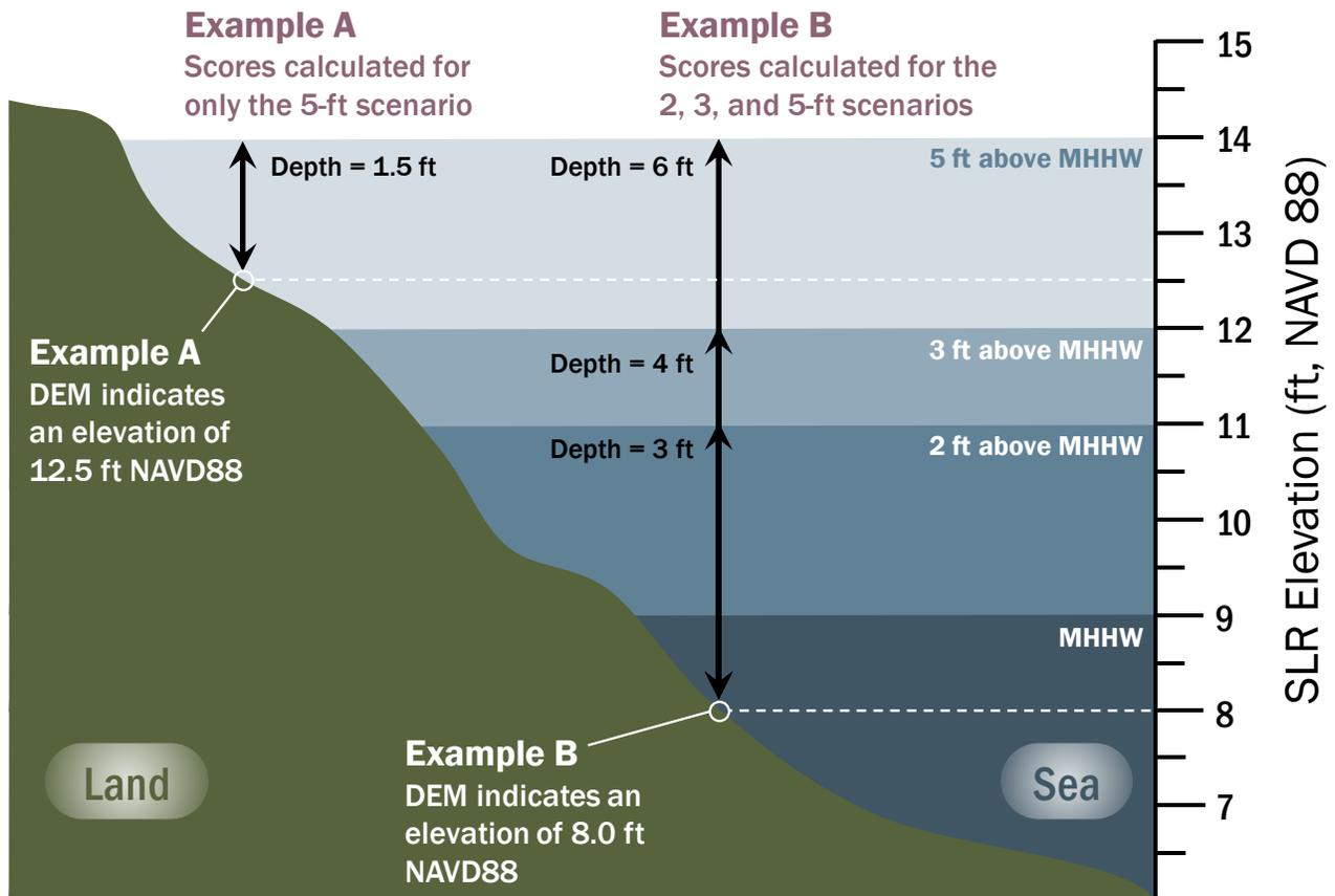
**Figure 3-5. Illustration of Depth Estimation for Each Sea Level Inundation Extent**
