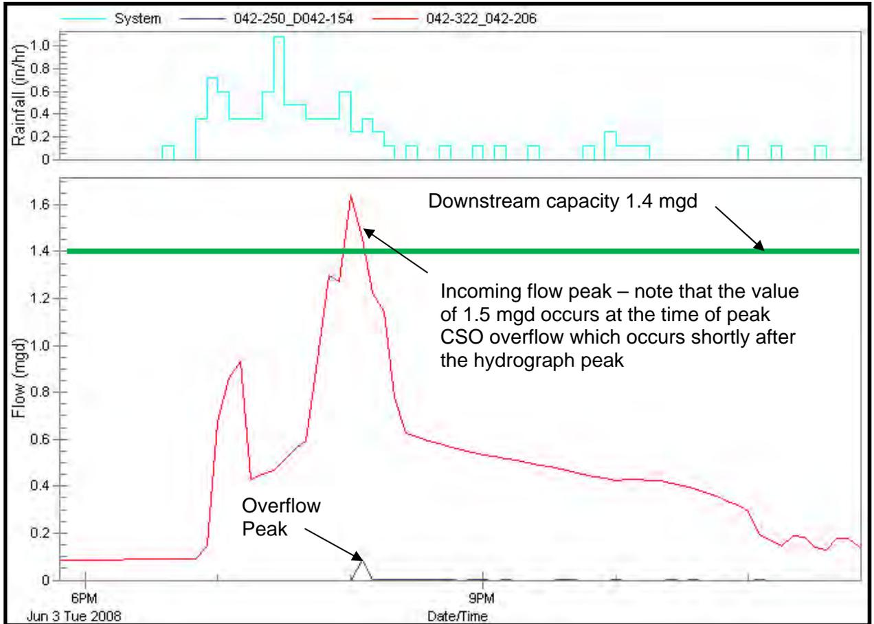
**Figure 2-2 Model output for the peak flow values at the NPDES 30 control structure during the control event.**
