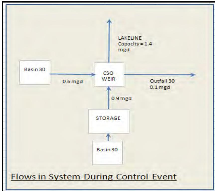
Figure 2-1 NPDES 30 flow schematic
