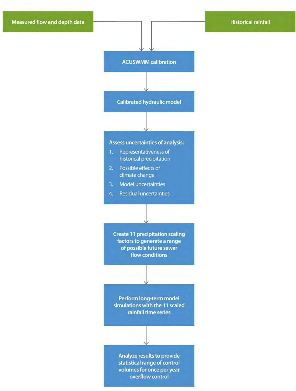
Figure 2. Process to develop control volumes
