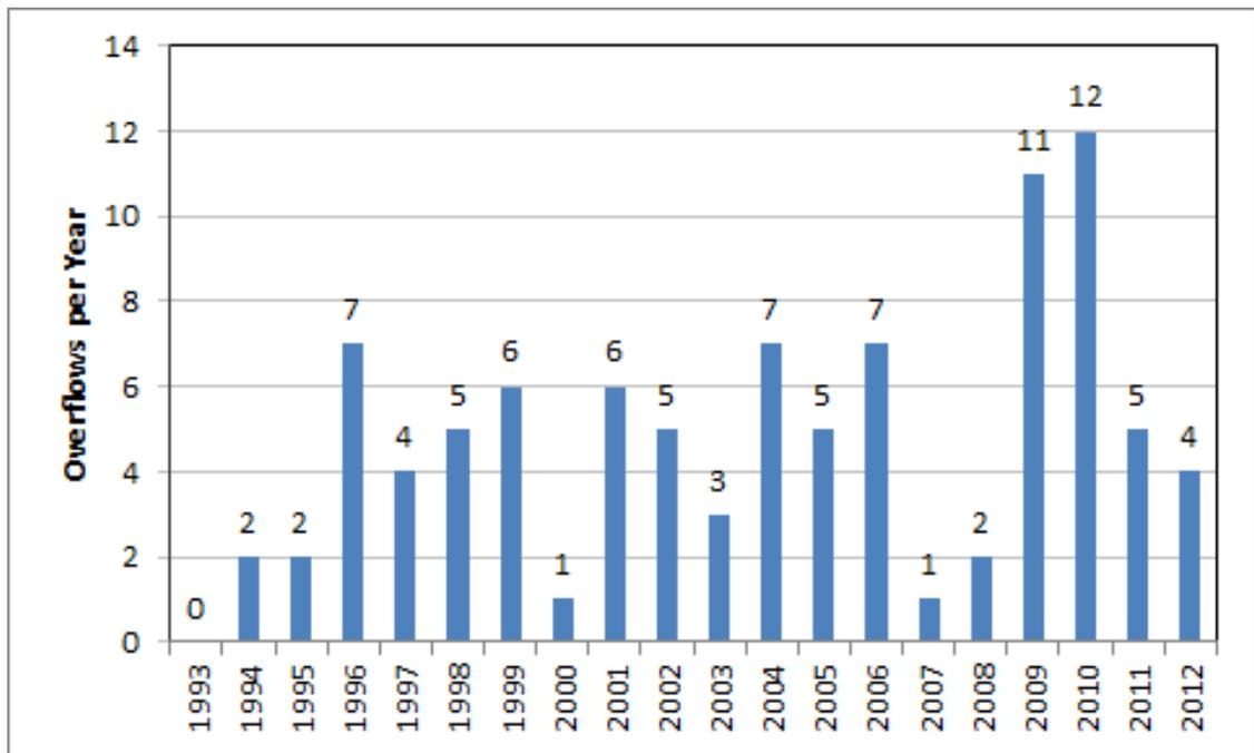
Figure 3-3. East Waterway overflow frequency per year from 1993 through 2012
