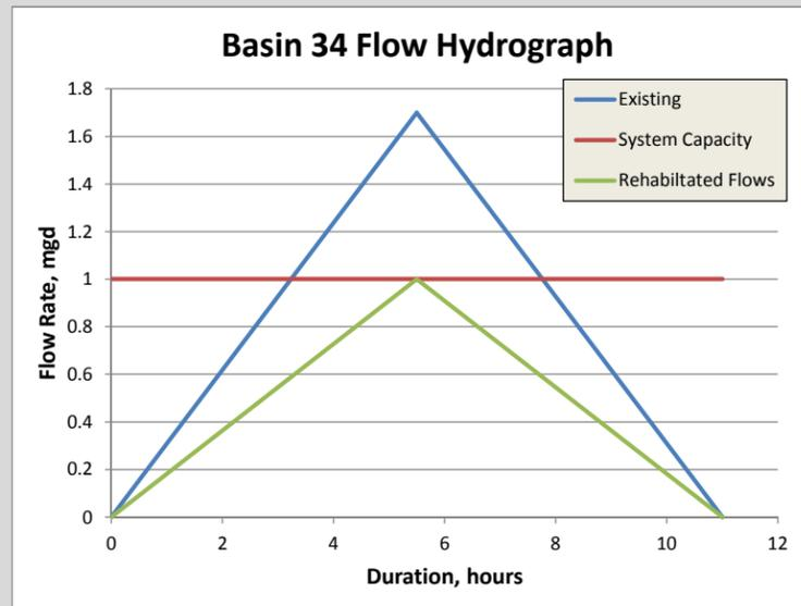
The flow above the System Capacity (red line) represents the overflow from the basin. The Existing (blue line) represents peak basin flows during the control event. The Rehabilitated Flows (green line) represents the remaining flows after the rehabilitation work is completed. Again, the remaining overflow is that portion that is above the red line.
