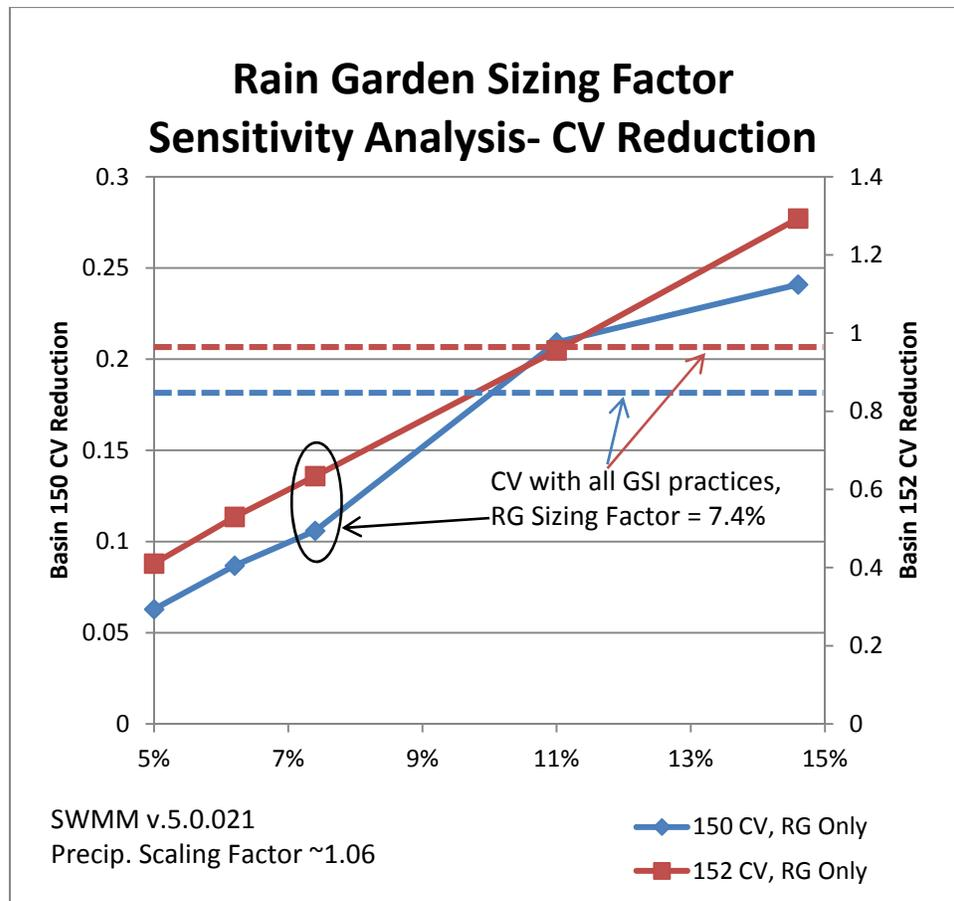
Figure 2. Raingarden Sizing Factor Sensitivity
