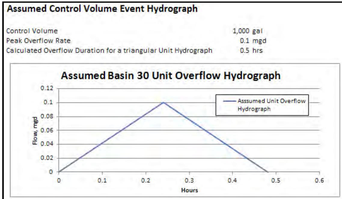
Figure 2-3 Unit hydrograph of NPDES 30 CSO Overflow
