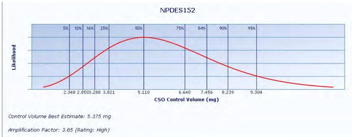
**Figure 1. Control volume best estimate, uncertainty bounds, and amplification factor for the Ballard 152 CSO Basin Overflow Structure**
