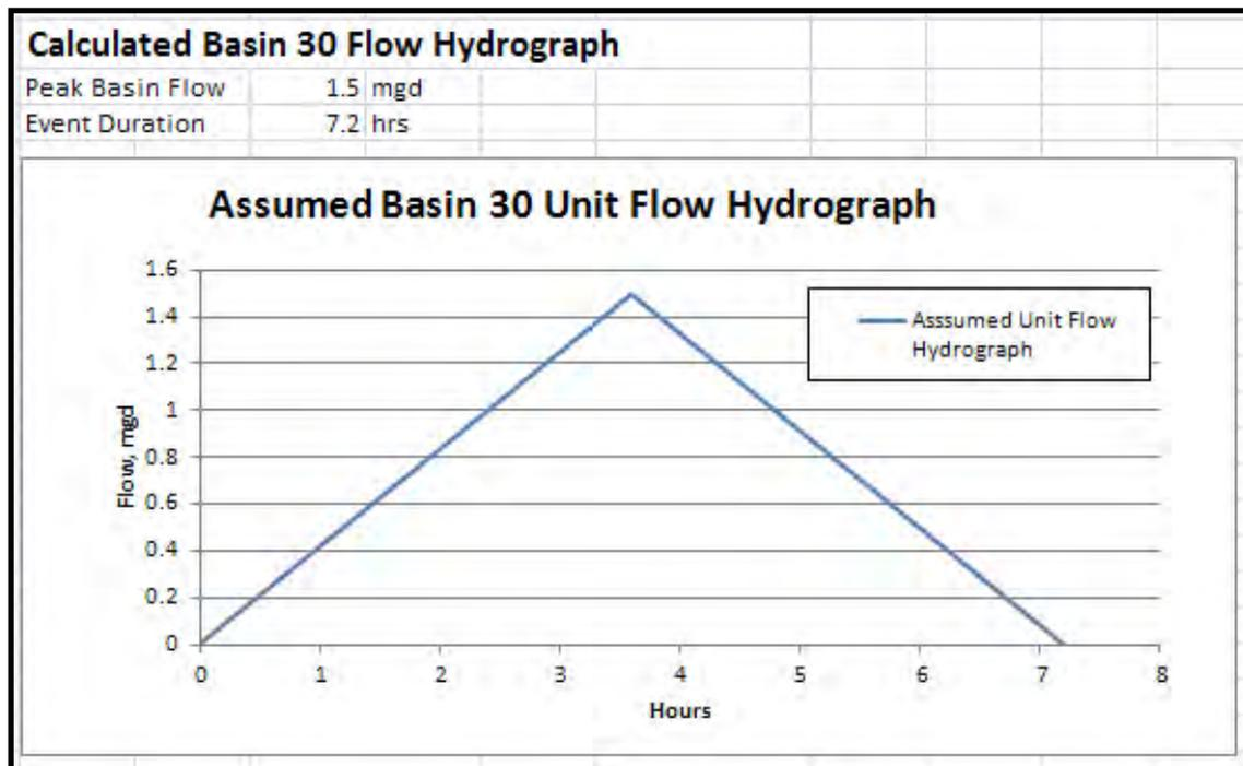
Figure 2-4 NPDES Basin 30 Hydrograph for the control event
