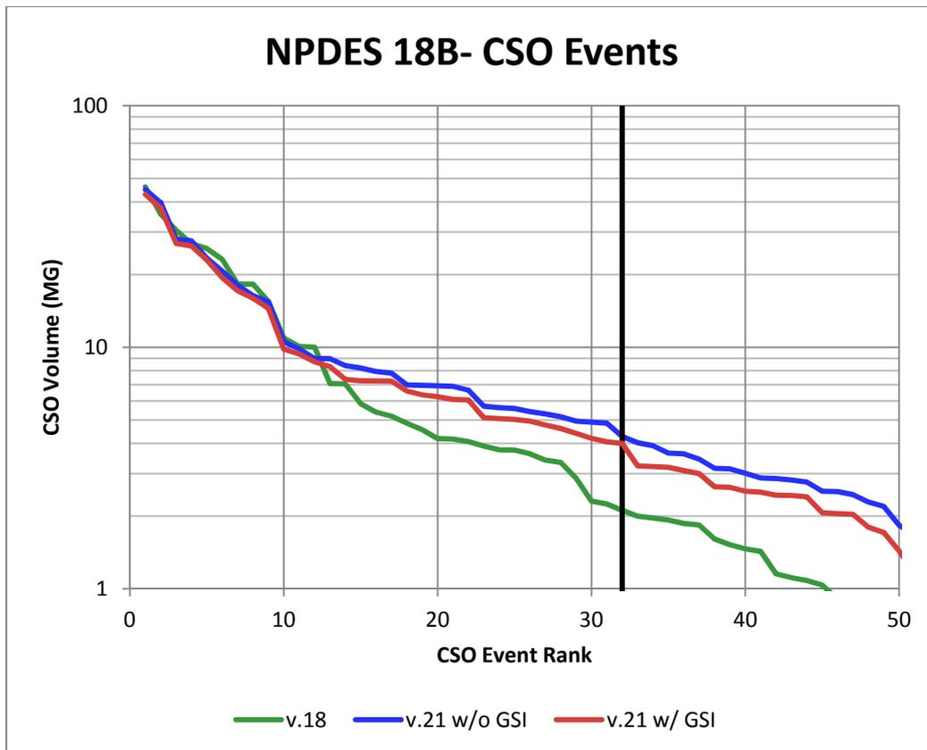
Figure 5. CSO Volume for the 50 largest events from each of the three model runs of the Basin 18B model. The 32<sup>nd</sup> ranked event in a 31-year simulation is considered the control volume.
