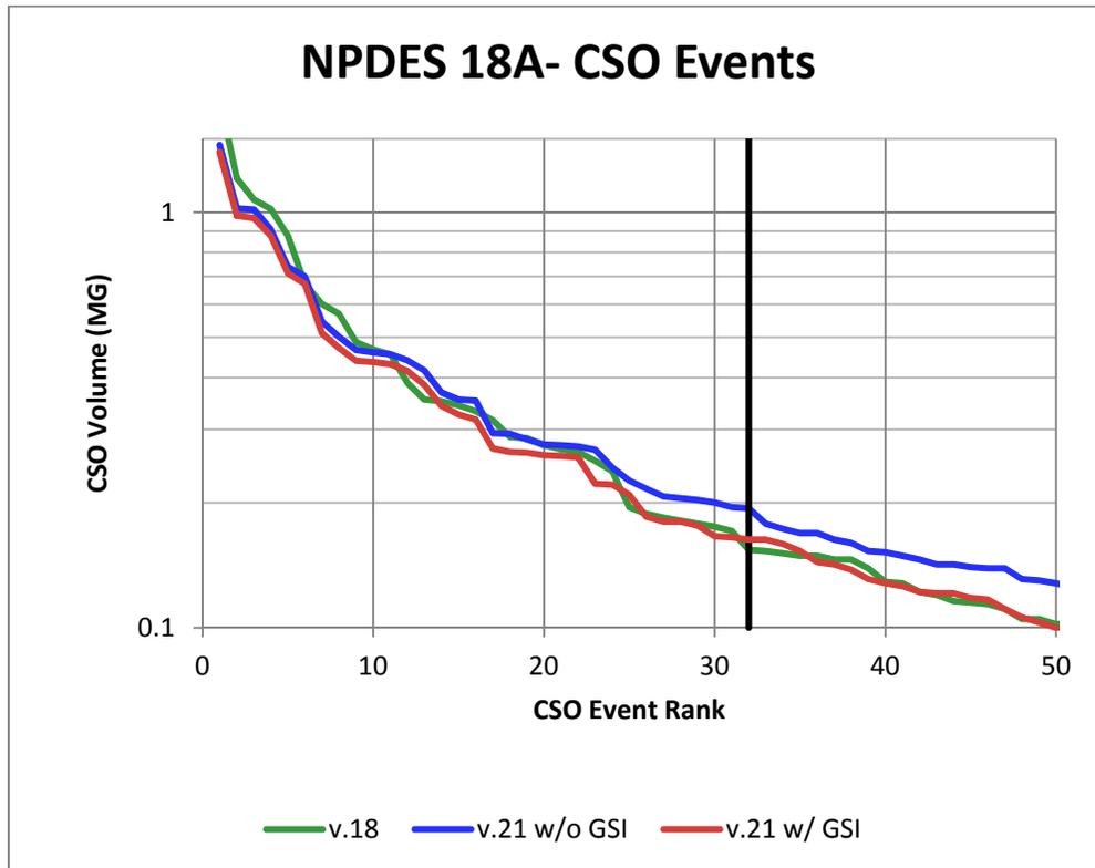
Figure 4. CSO Volume for the 50 largest events from each of the three model runs of the Basin 18A model. The 32<sup>nd</sup> ranked event in a 31-year simulation is considered the control volume.
