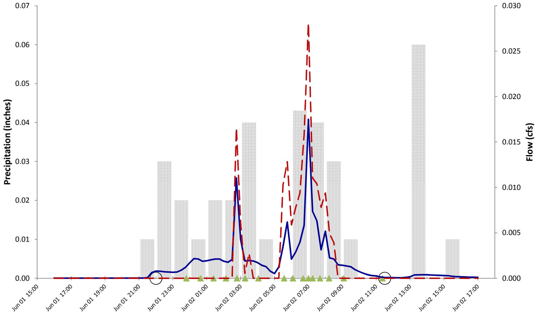
■ Precipitation    ○ Event (Start/End)    ▲ Sample Aliquot    △ Sample Missed    — Flow    - - Bypass Flow
