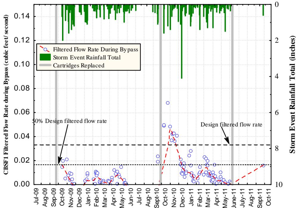
Figure 5.3.5b. CBSF2 Temporal Plot of Treated Flow Rate and Precipitation Depth
