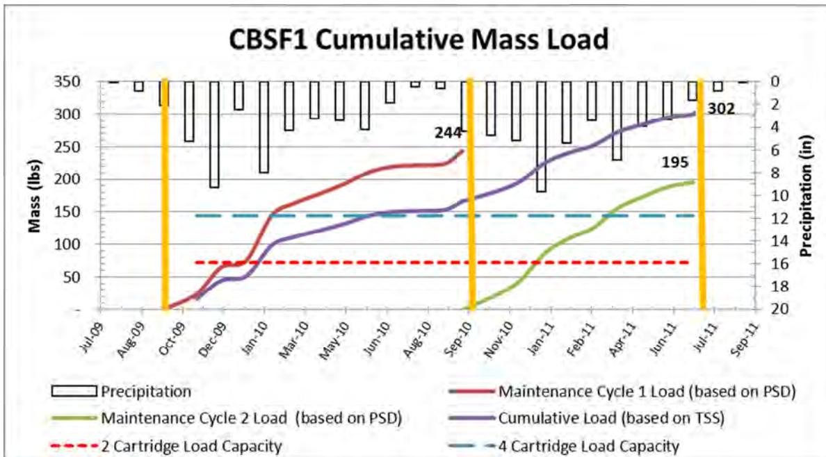
Figure 1. Estimated cumulative mass load received by CBSF1.
