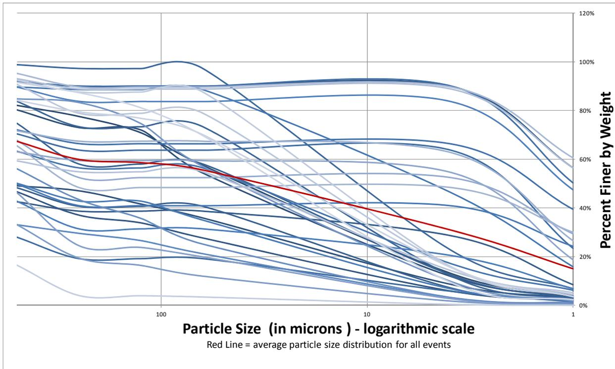
Figure 4.2.1c. Effluent Particle Size Distribution Data – All Events
