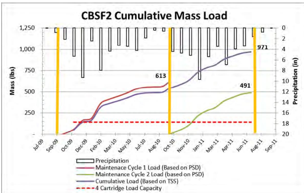
Figure 2. Estimated cumulative mass load received by CBSF2.
