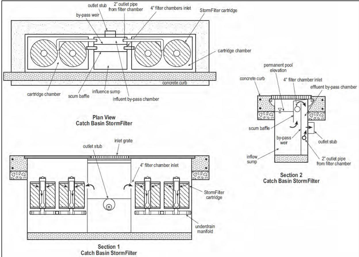
The monitored CBSFs were sized using the Western Washington Hydrology Model Version 3 (WWHM3), an Ecology-approved continuous runoff model. The units were sized assuming an online, or flow-through facility, based on the manufacturer’s recommendation and the definition provided in the Stormwater Management Manual for Western Washington (Ecology 2005), Section 4.5 Hydraulic Structures, 5.1 Flow Splitter Designs:
