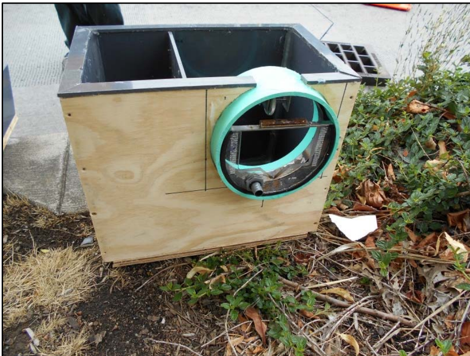
Figure 9. Weir box (prior to installation).
