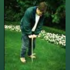
Digging in is the only way to determine soil depth. A core-sampler makes checking soil depth and moisture easy.
