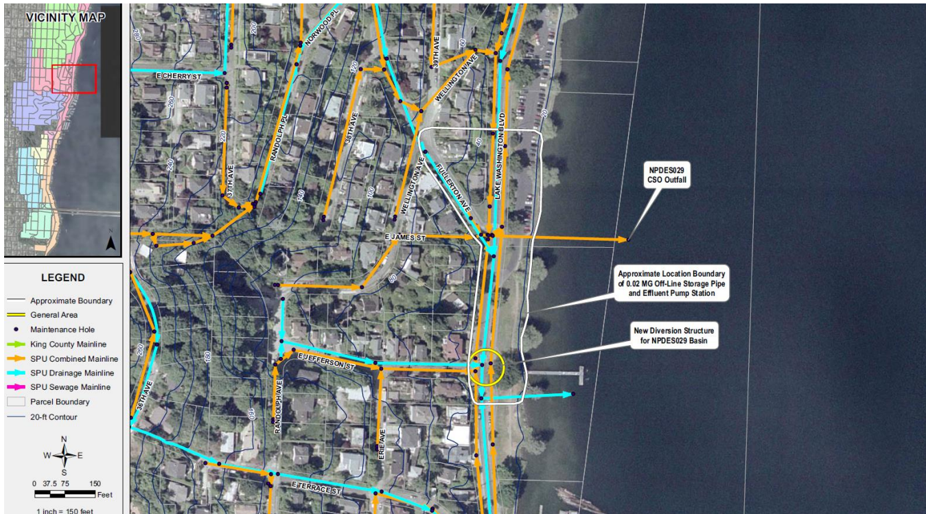
Figure 5-22. CSO Outfall 029 Recommended Control Measure
