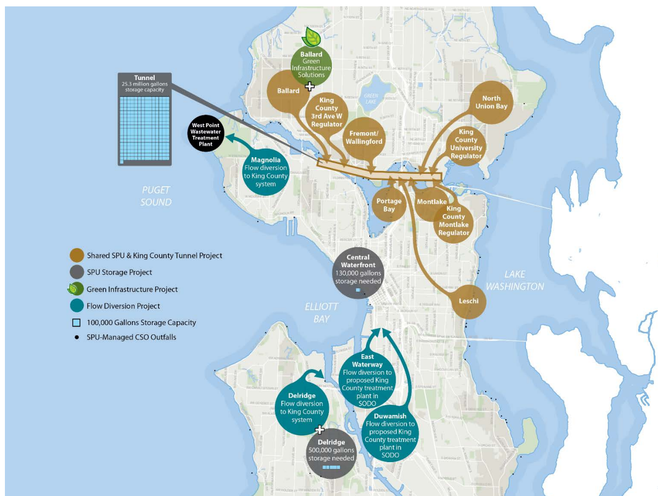
Figure 3-20. Shared Ship Canal Tunnel Option
