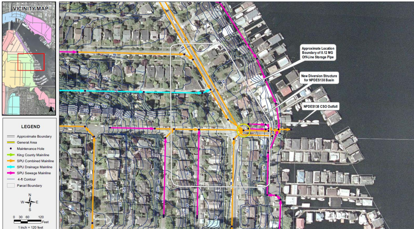
Figure 5-25. Portage Bay/Lake Union CSO Outfall 138 Recommended Control Measure
