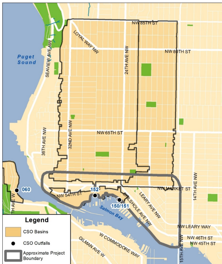
Figure 3-2. Ballard CSO Area Boundaries, CSO Outfall Locations, and General Area for Potential CSO Control Measure Implementation
