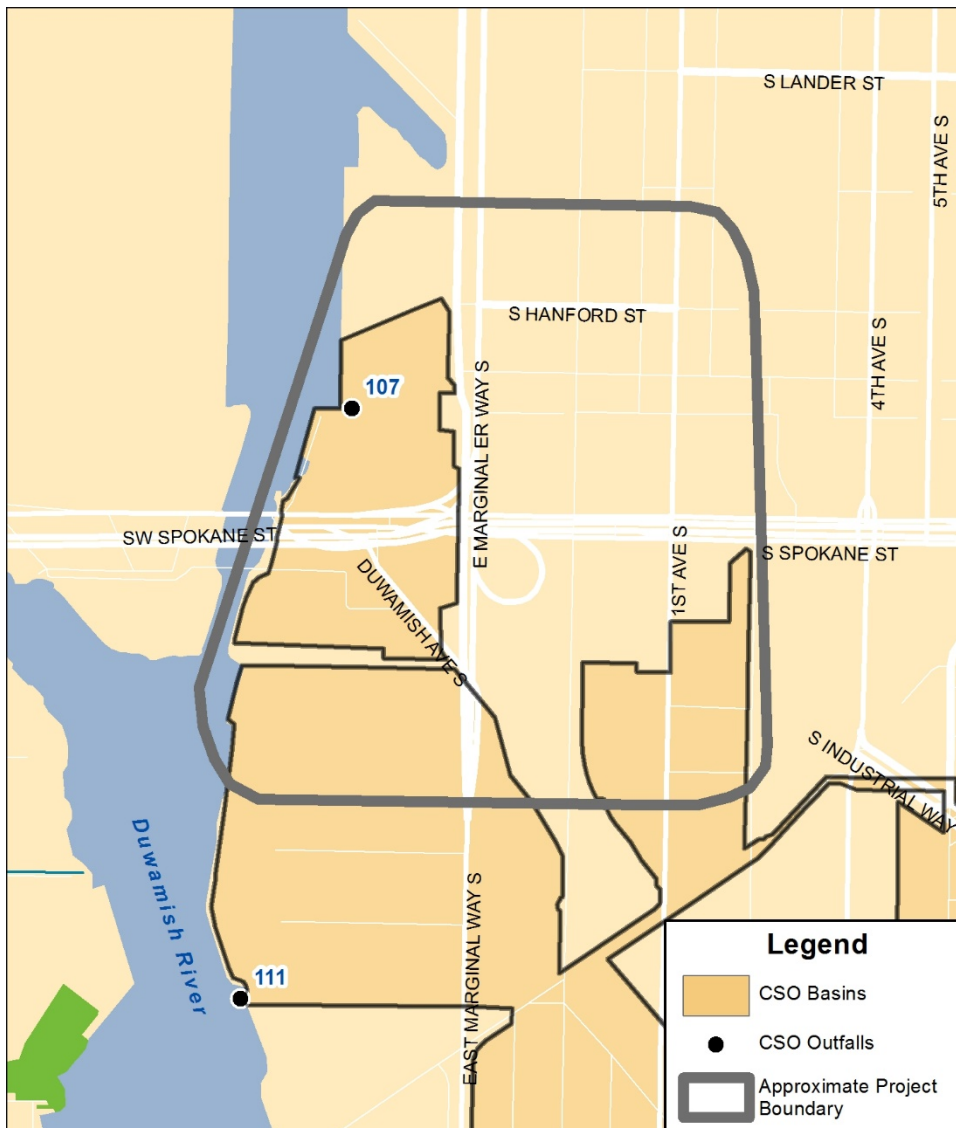
Figure 3-8. East Waterway CSO Boundaries, CSO Outfall Locations, and General Area for Potential CSO Control Measure Implementation
