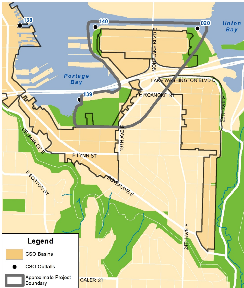
Figure 3-10. Montlake CSO Boundaries, CSO Outfall Locations, and General Area for Potential CSO Control Measure Implementation
