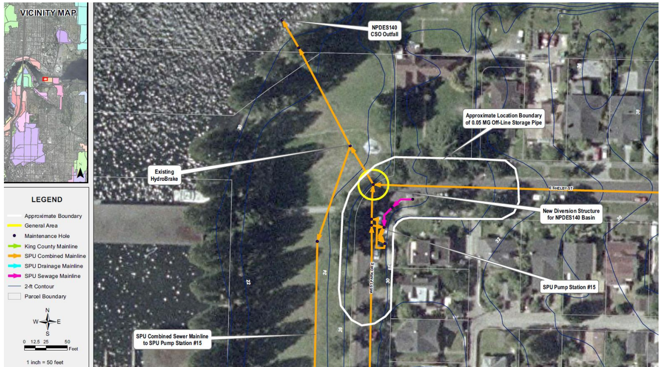
Figure 5-19 CSO Outfall 140 Recommended Control Measure
