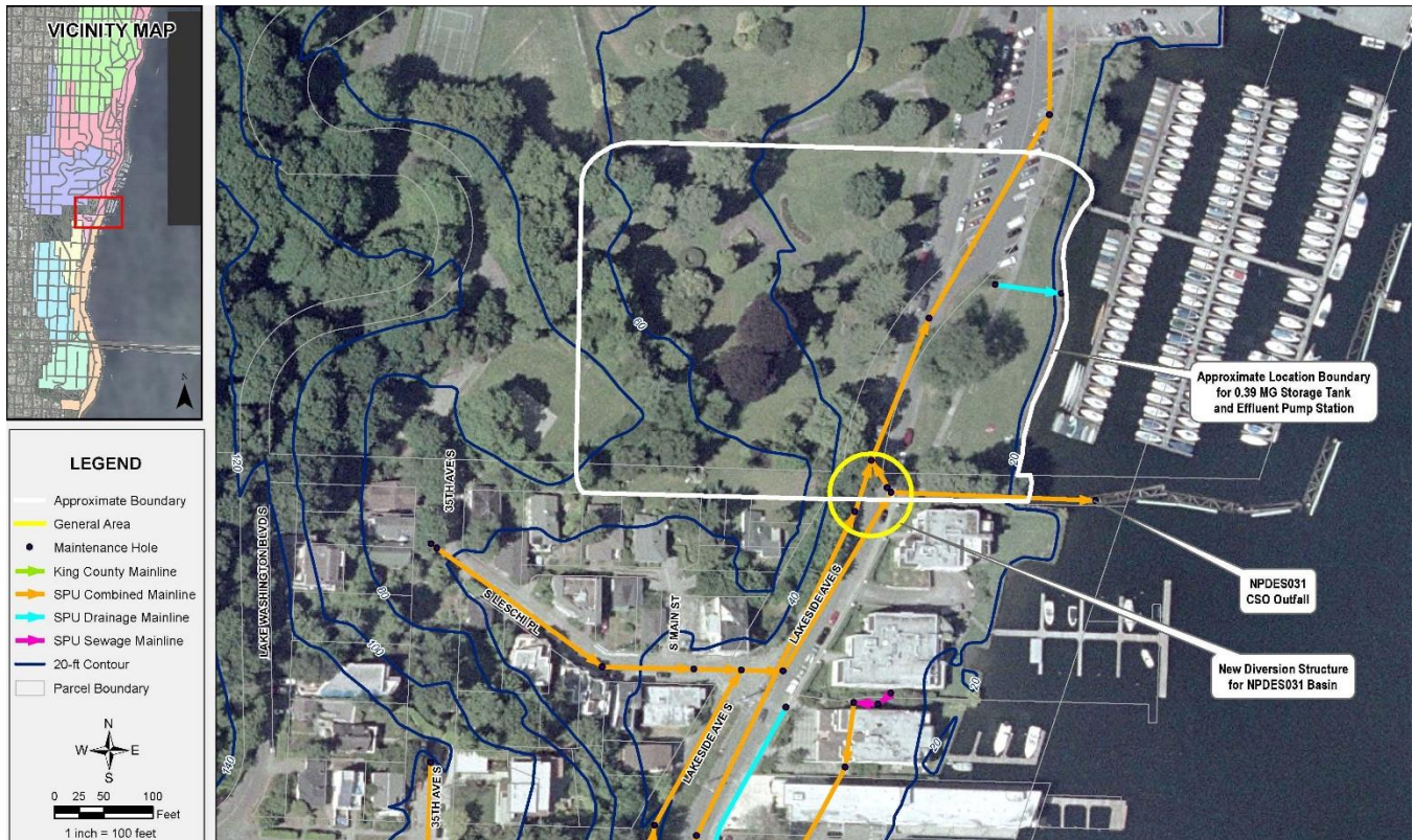
Figure 5-23. CSO Outfall 031 and 032 Recommended Control Measure
