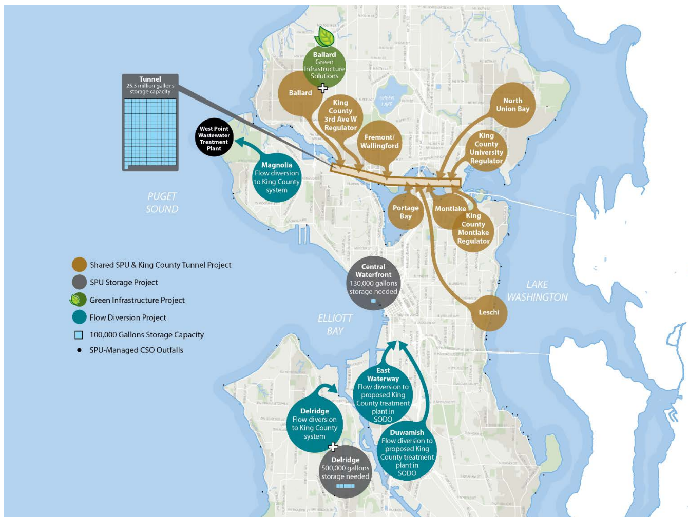
Figure 3-20. Shared Ship Canal Tunnel Option
