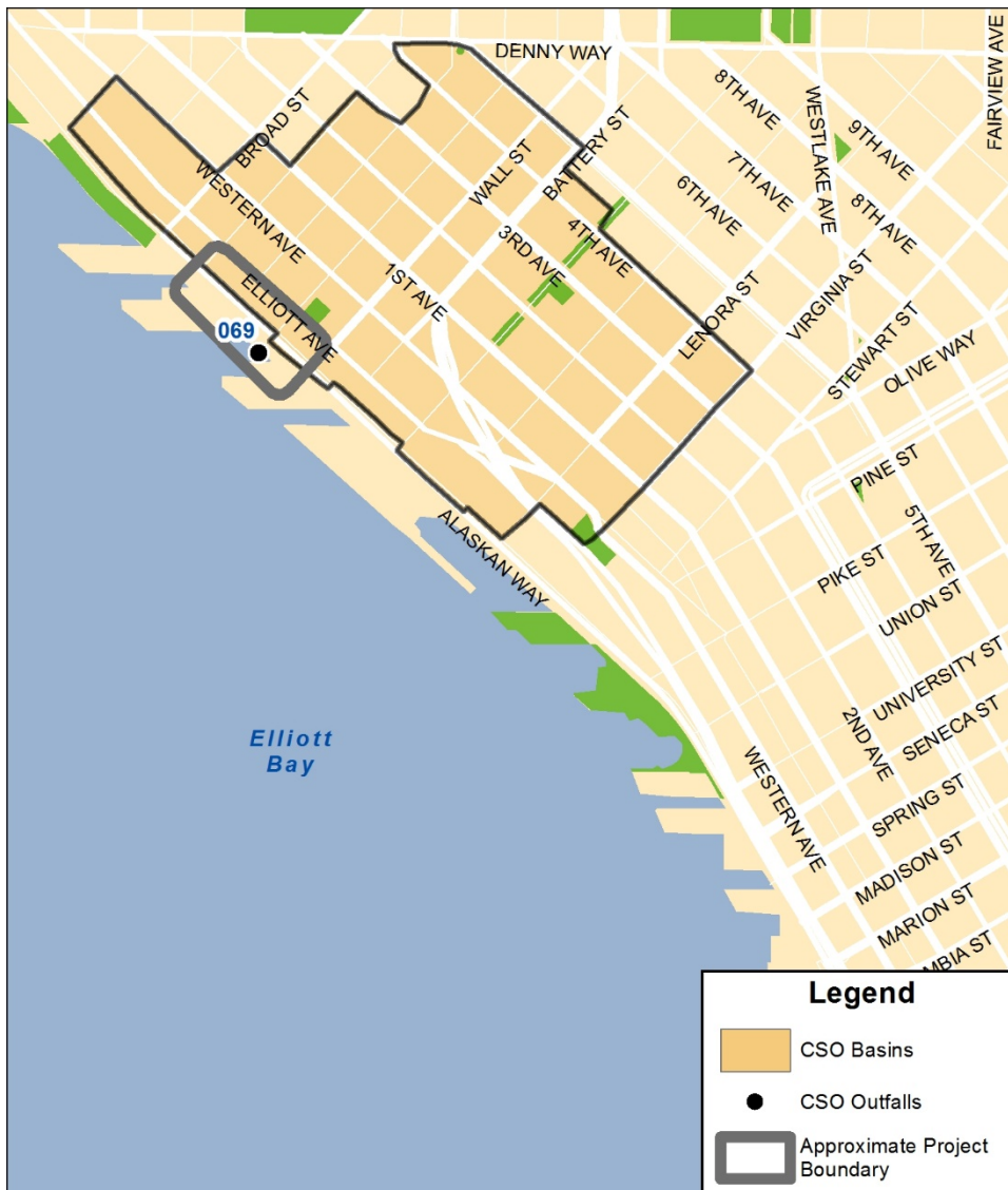
Figure 3-5. Central Waterfront CSO Boundaries, CSO Outfall Locations, and General Area for Potential CSO Control Measure Implementation
