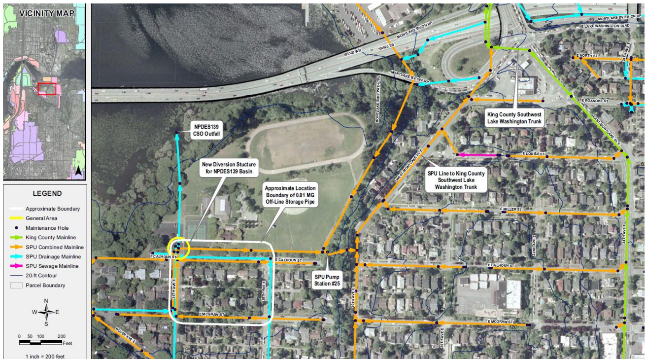
Figure 5-18 CSO Outfall 139 Recommended Control Measure
