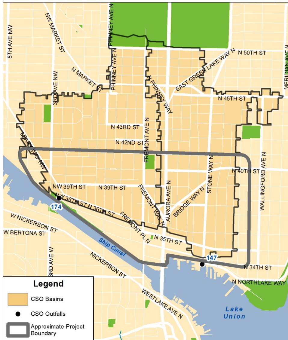
Figure 3-6. Fremont/Wallingford CSO Boundaries, CSO Outfall Locations, and General Area for Potential CSO Control Measure Implementation
