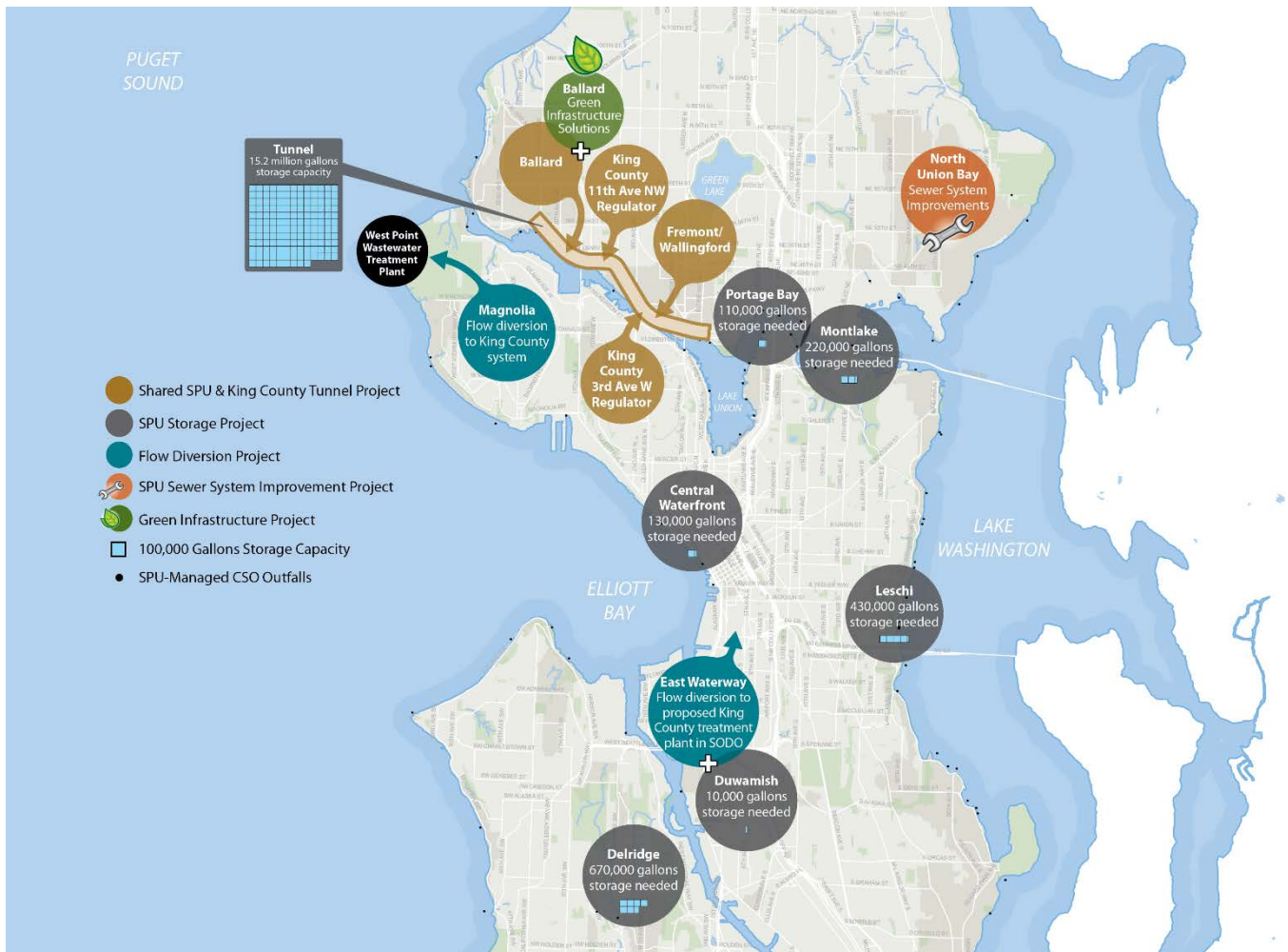
Figure 3-19. Shared West Ship Canal Tunnel Option
