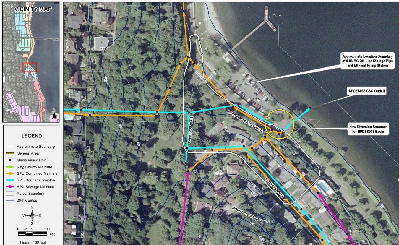
Figure 5-24. CSO Outfall 036 Recommended Control Measure
