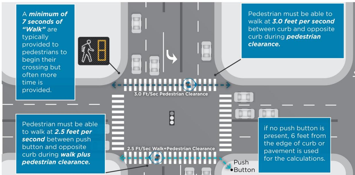
Figure 2: Pedestrian Interval Requirements Based on Walking Speed
