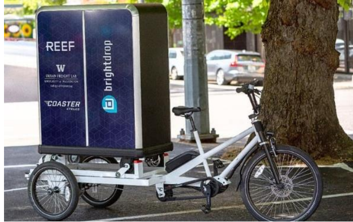
Electric pallet used for goods delivery
