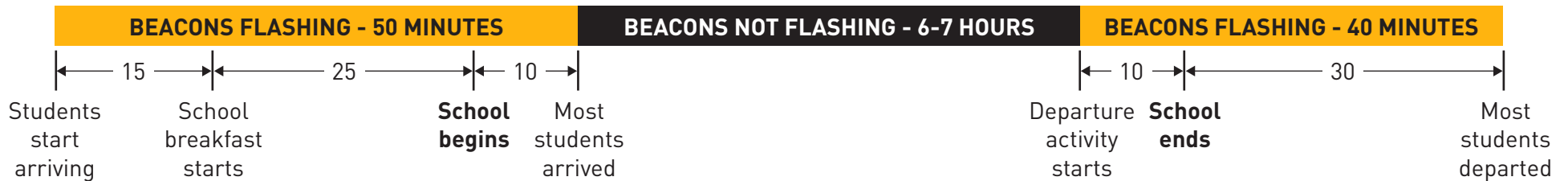
Figure 1 – Typical school flashing beacon schedule
