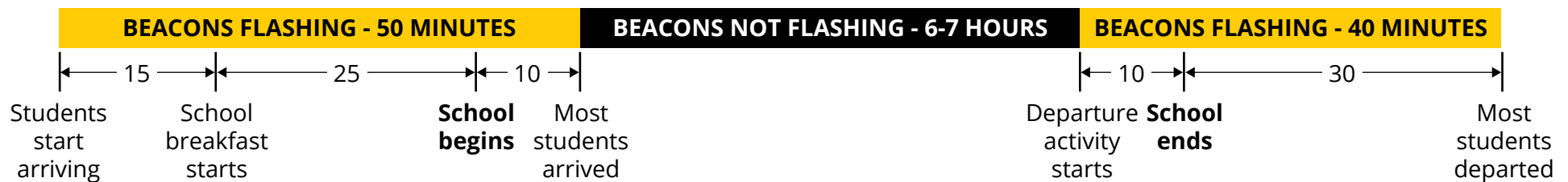
Figure 1 – Typical school flashing beacon schedule
