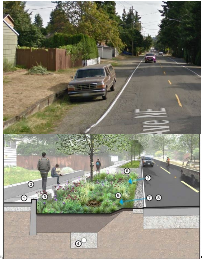
Figure 1: Sidewalk and Natural Drainage System Project
