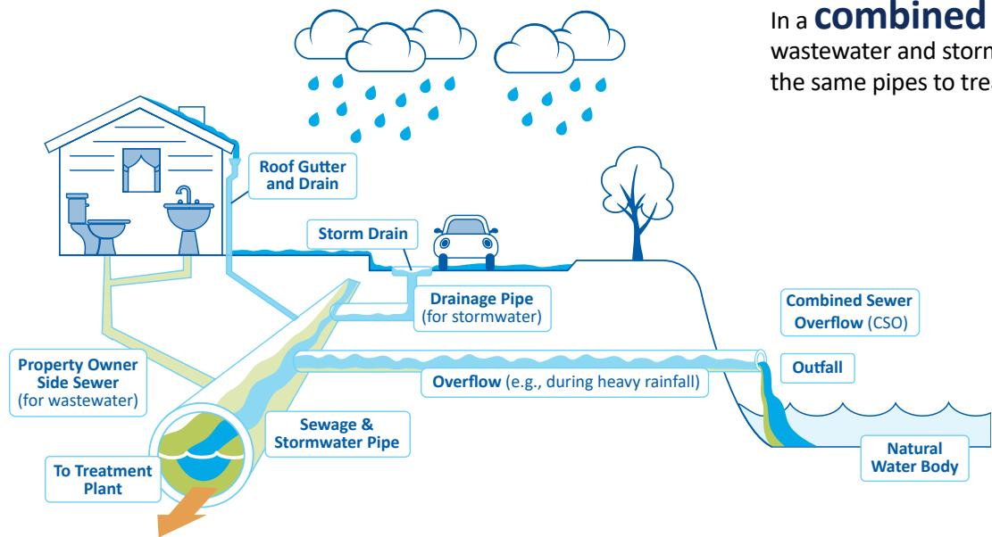
In a **combined sewer system**, wastewater and stormwater travel in the same pipes to treatment plants.
