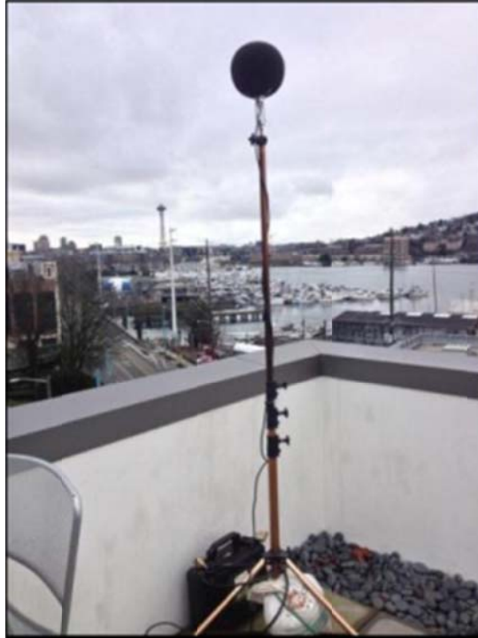
Photo 5 – Typical Ambient Vibration Monitoring Station
