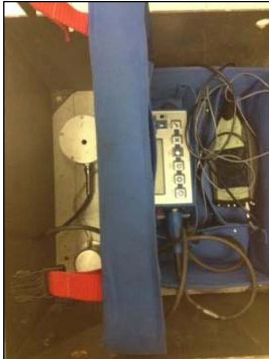
Photo 5 – Typical Ambient Vibration Monitoring Station
