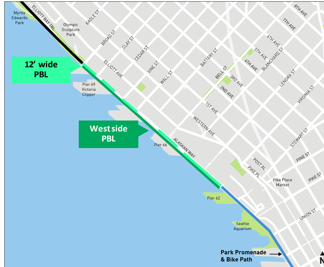
Continuous 10' two-way PBL on the west side of Alaskan Way, with segments that expand to 12' in width.
