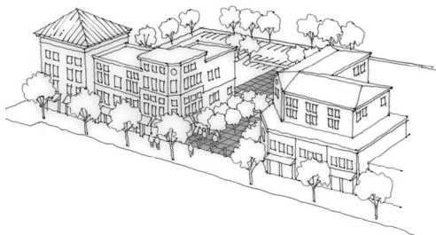
An example of a parking area designed to serve both parking and pedestrian needs with unit pavers, landscape and bollards.
