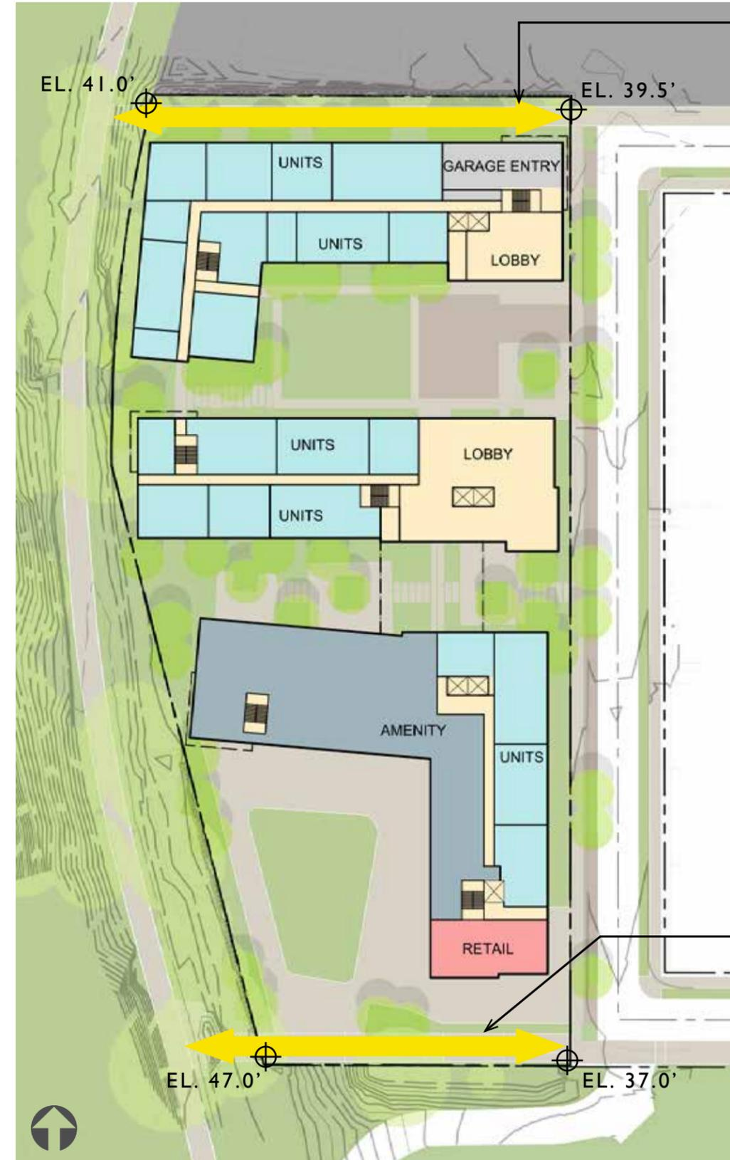
NORTHERN TRAIL CONNECTION FOR PEDESTRIANS - COMPOSED OF ADA ACCESSIBLE RAMPS WITH LESS THAN 5% GRADE
