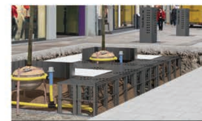
Proposed benefit #4: Silva Cells promote tree growth and treat stormwater
