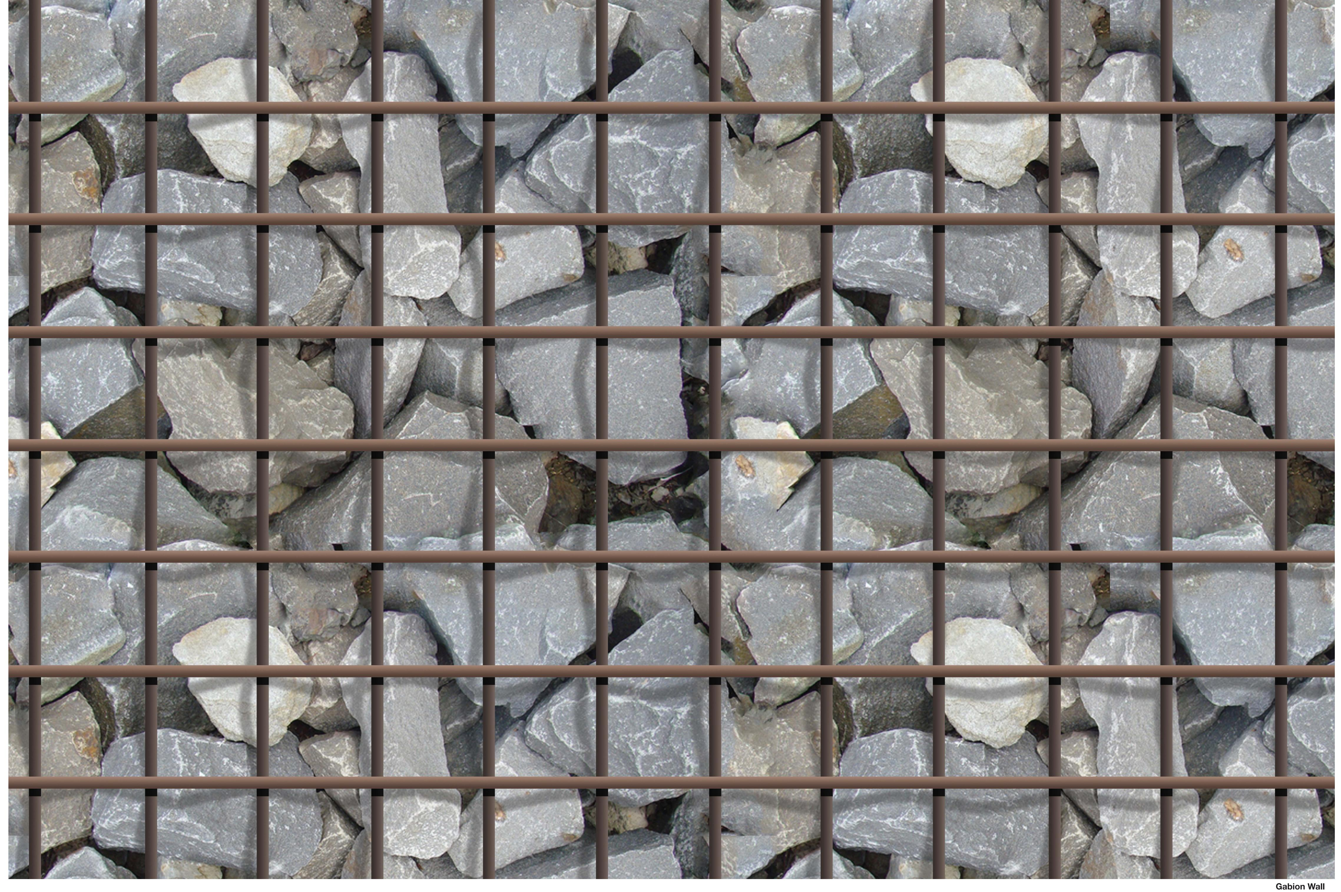
Full Scale Virtual Mockup 4" to 8" Basalt Fill with 3/8" Wire at 4" On Center
