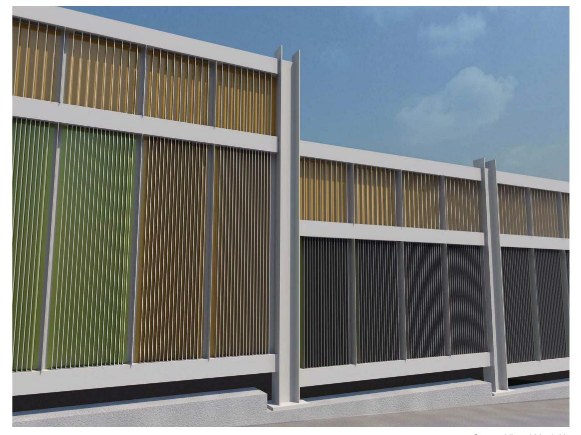
Screen Virtual Mock Up Painted Steel Structure with Aluminum Bar Grating and Colored Acrylic Panels
