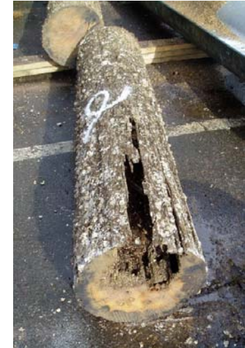
Timber pile from Colman Dock that has been removed and replaced due to deterioration.
