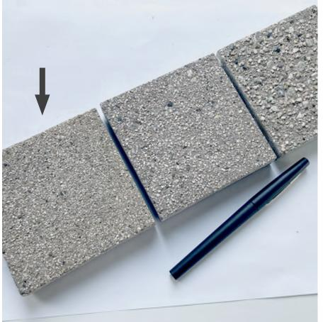
Plain concrete (no color). Lightly exposed aggregate surface finish.
