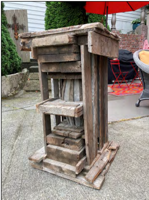
Fig. 26 – Mold used by Fausto Cettolin to form columns.
