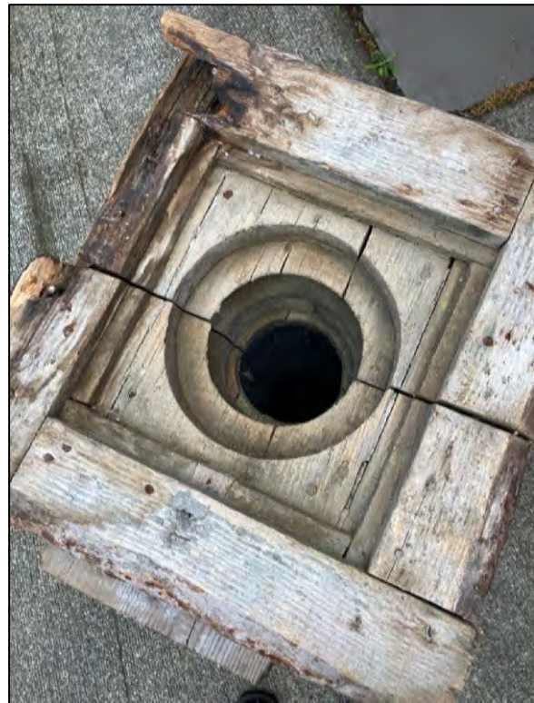
Fig. 26 – Mold used by Fausto Cettolin to form columns.
