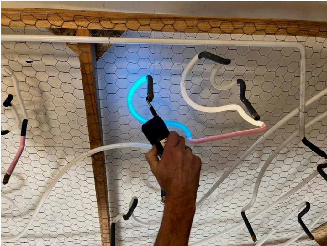
Figure 10. Below, testing the tube light color on the sign's eyebrow piece.
