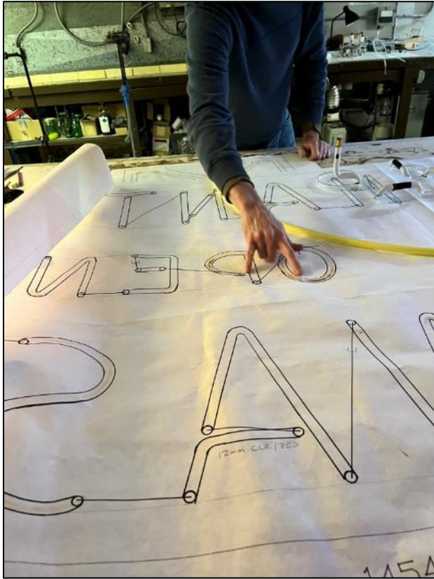
Figure 11 Left, the full scale template for the neon tube letters
