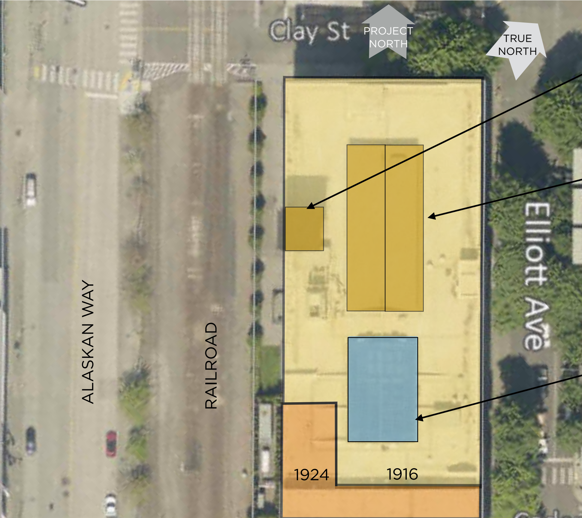
1916 CLEARSTORY ROOF Butterfly section w/ thin concrete roof & parapet
