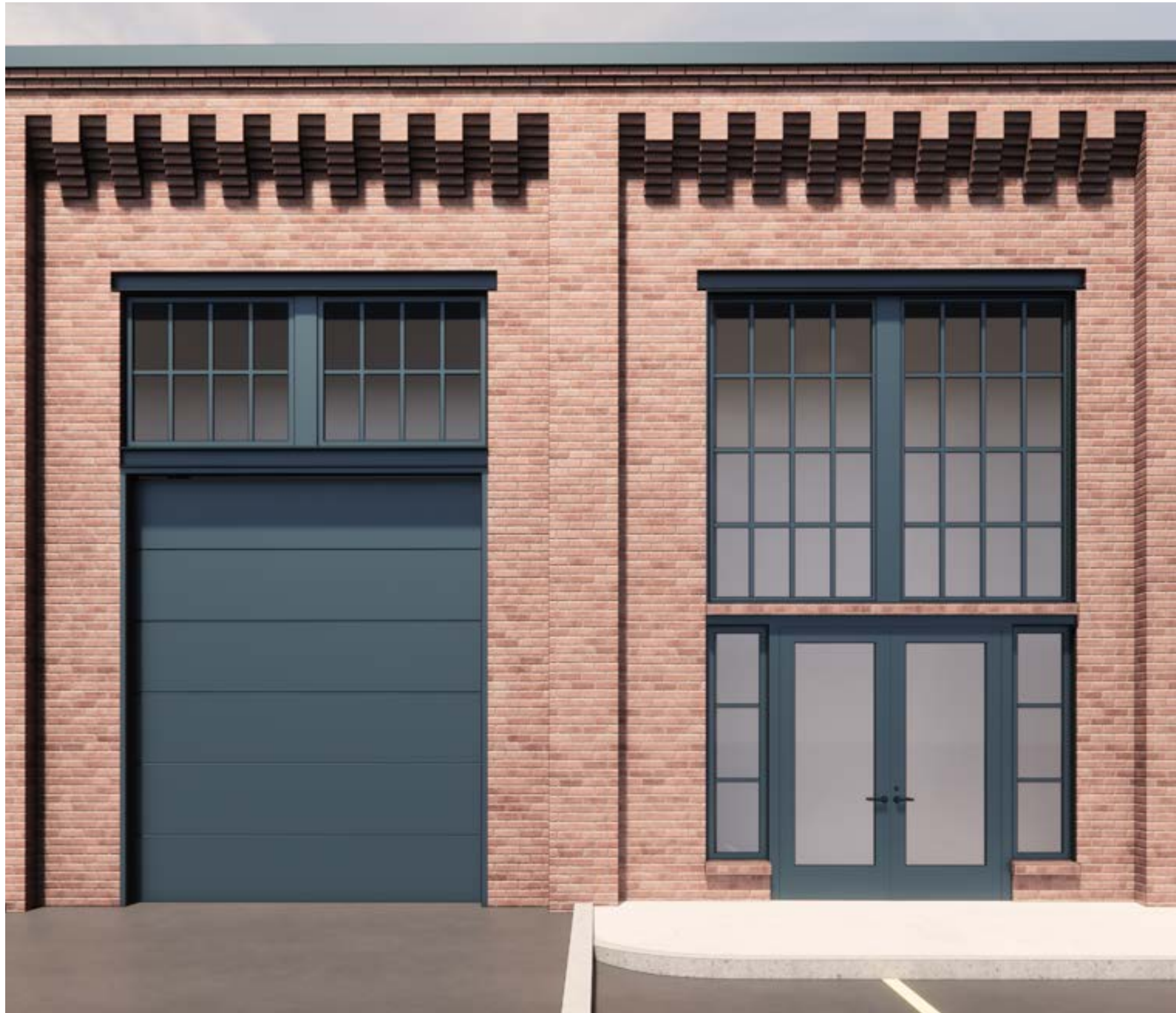
STUDY 5 per ARC Request Retain brick at sidelights only - add brick sill.
