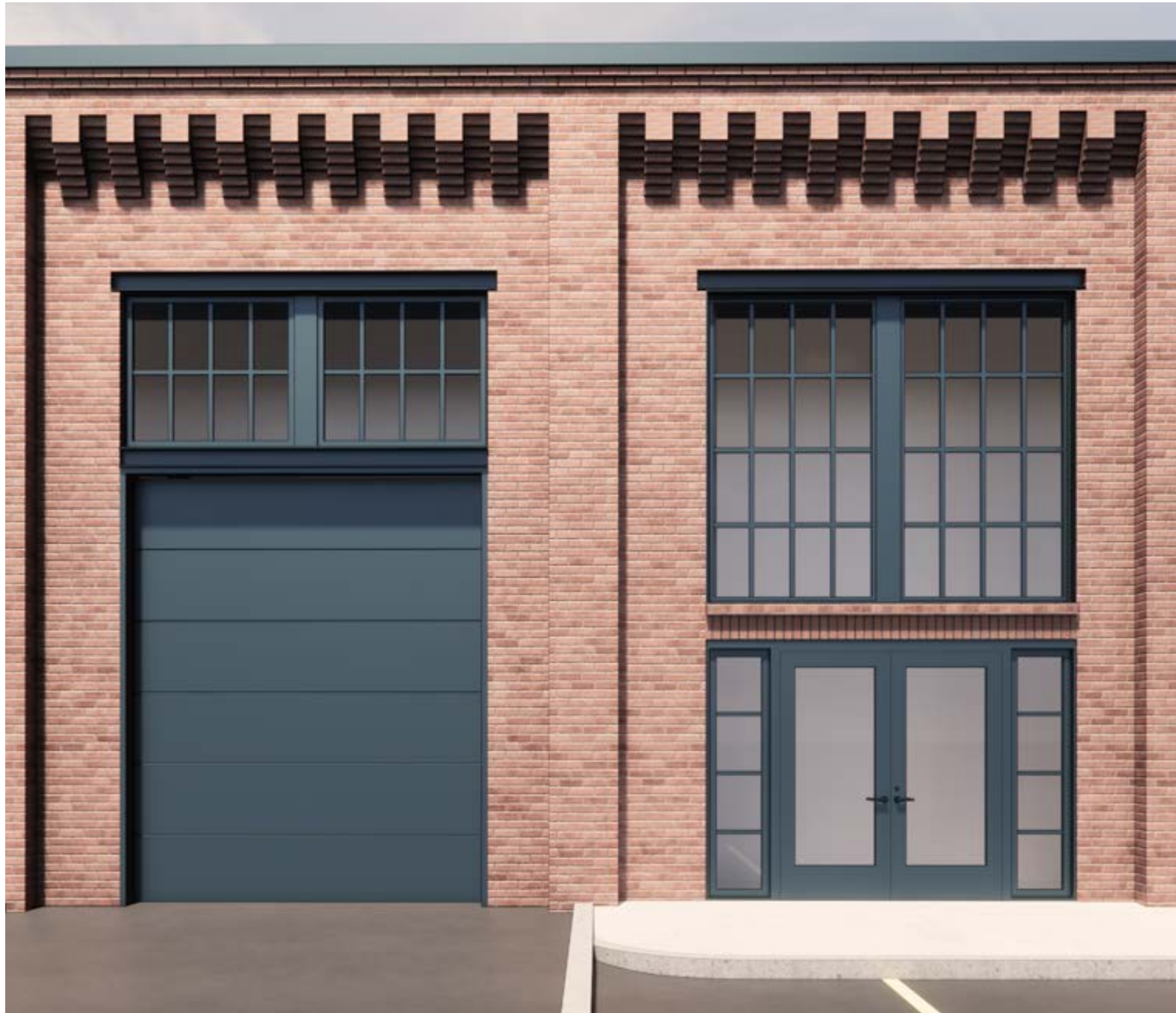
STUDY 2 per ARC Request Retain Brick at Window Sill - Soldier Course Added
