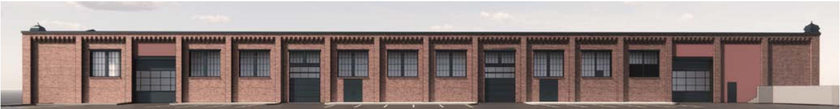
ALT 1 - REMOVE SIDELIGHTS & ADD GLAZING TO TOP OF OVERHEAD DOORS
