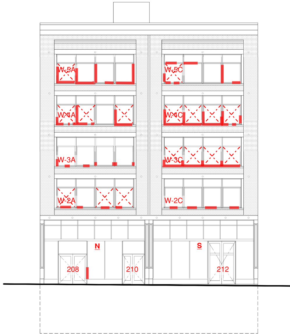
Diagram showing surveyed window locations on west elevation of 210 Third Avenue South.
