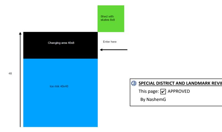
There are no attachments to the ground. The synthetic ice rink will sit on plywood sheeting as to not harm the bricks in the park.
