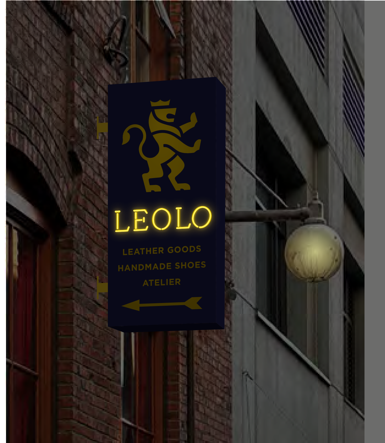
SIGN 2: NIGHT VIEW NOTE: SIGN IS ATTACHED WITH QTY 4 . EPOXY SET .5" X 6" ALL-THREAD UNITS WITH 1" WASHERS AND NUTS
