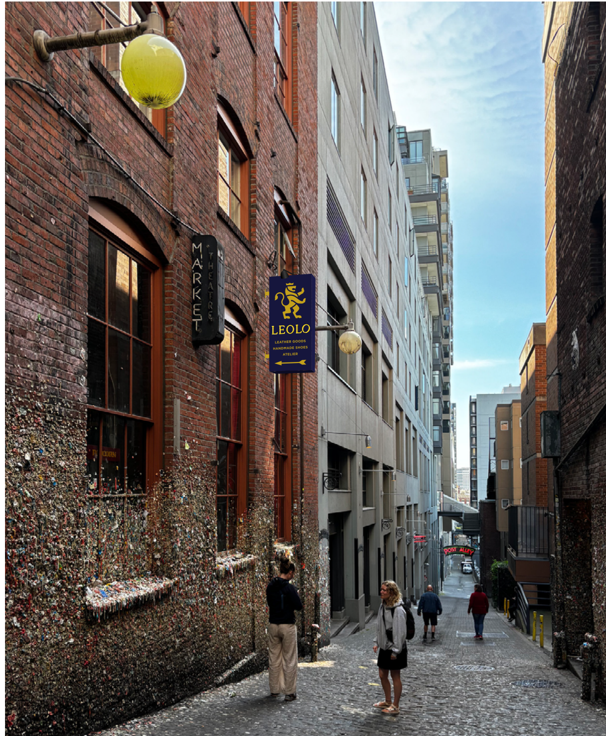
SIGN 2: 24"X51"X8" DOUBLE SIDED NEON SIGN W/ HANDPAINTED (USE PAINT MASK) LOGO, LETTERING AND ARROW, "LEOLO" LETTERING IS 4.5" TALL
