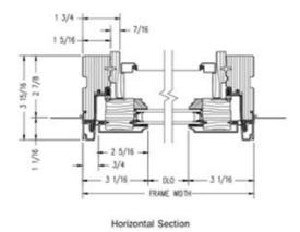
**Detailed section of clad window units**
