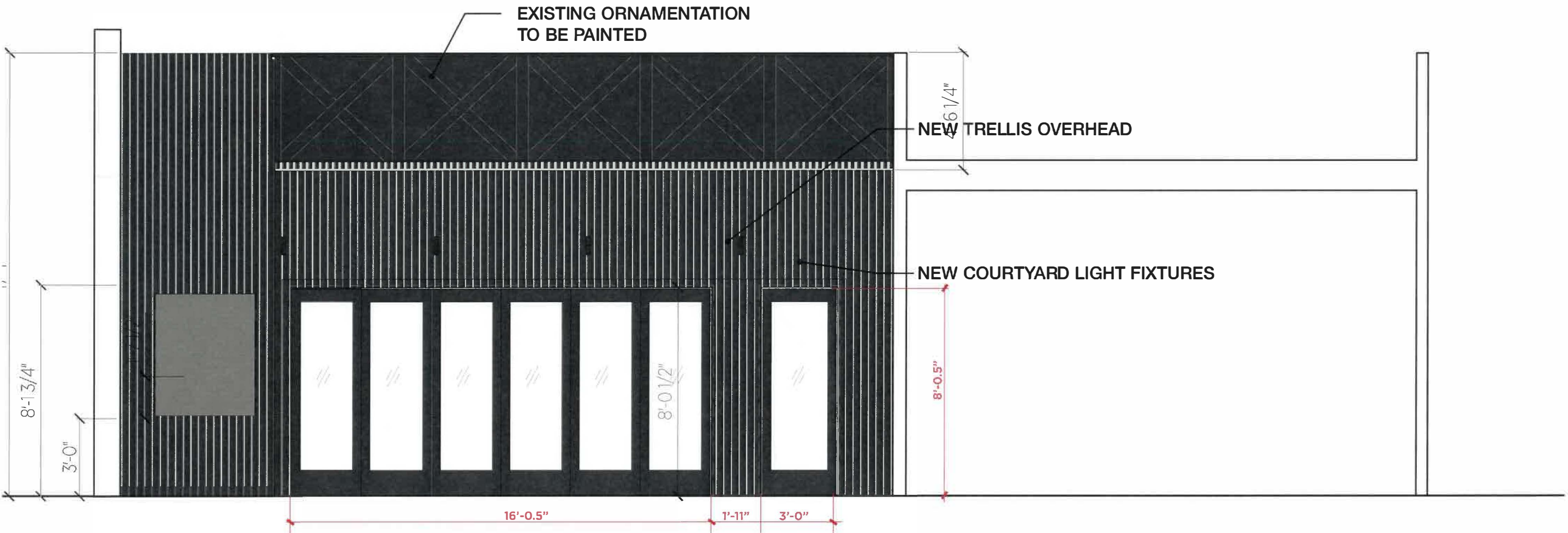
1 NEW EAST ELEVATION (Courtyard Only) 1/4" = 1'-0"
